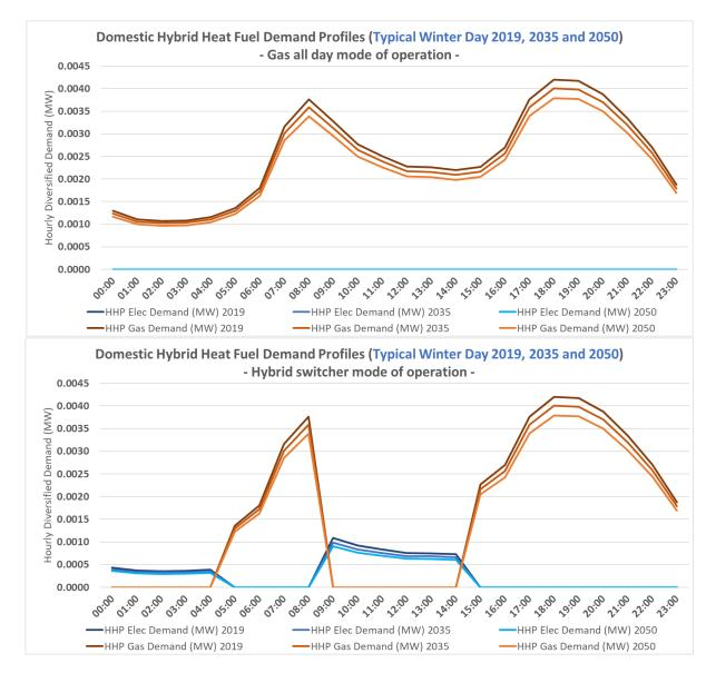
Figure 5-9 Diversified hybrid heat fuel demand profiles used in seasonal day modelling, reflecting several aggregated properties and converted to a single house profile
