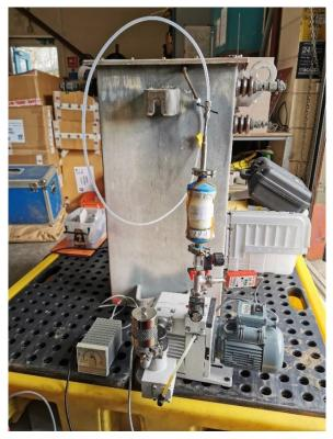
Fig.8 Experimental setup using a test transformer with ~50 ppm PCB contamination.
