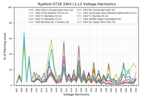
Figure 2-3: 95th percentile aggregate voltage harmonic values for the Ryeford (GT1B) 33 kV sites calculated using all available data
