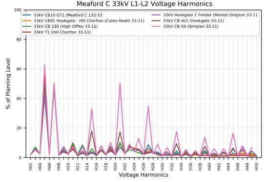
Figure 2-1: 95th percentile aggregate voltage harmonic values for the Meaford C 33 kV sites calculated using all available data
