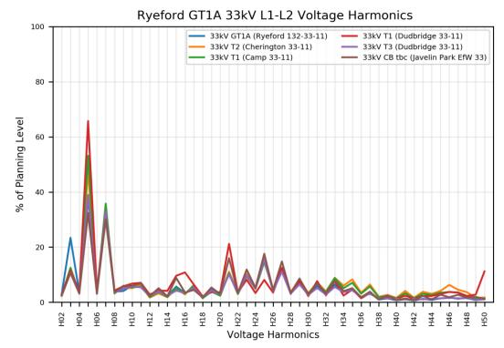
Figure 2-2: 95th percentile aggregate voltage harmonic values for the Ryeford (GT1A) 33 kV sites calculated using all available data
