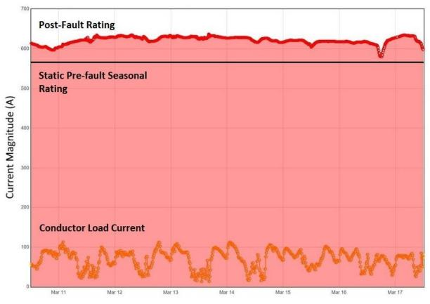
Figure 2-3 – Post-fault rating determined at trial site #241 (132kV K-Line)
