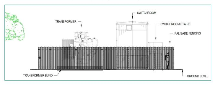
Figure 2-8 Pre-planning application substation elevation
