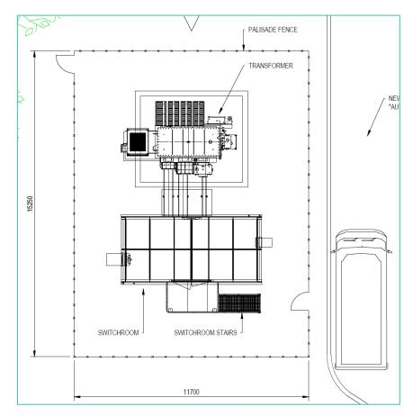
Figure 2-7 Pre-planning application substation plan
