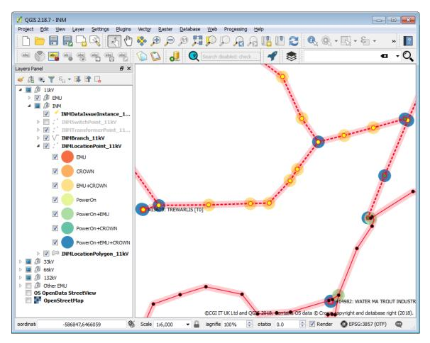
Figure 9 - Matched 11kV network example
