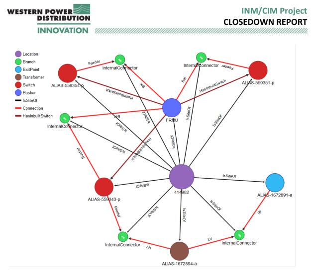
Figure 8 - Secondary substation PowerOn data example
