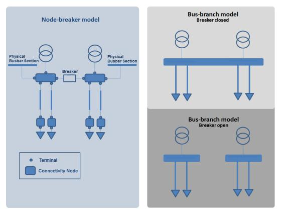
Figure 2 - Node-breaker vs bus-branch models
