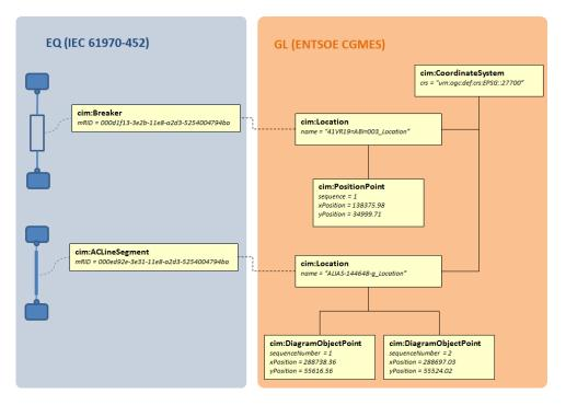
Figure 6 - Location objects in CIM GL file linked to CIM EQ conducting equipment
