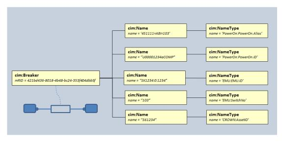
Figure 5 - Names associated with a circuit breaker in a CIM EQ file
