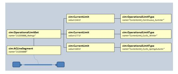
Figure 4 - Operational limits associated with AC line segment in a CIM EQ file
