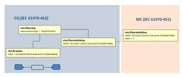
Figure 3 - Discrete measurement linked to circuit breaker in a CIM EQ file
