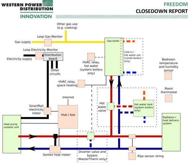
Figure 10: Schematic diagram of physical equipment deployed in a Freedom installation. Note: that the Daikin configuration is different as the boiler and heat pump have a "series" plumbing arrangement within the integrated unit.
