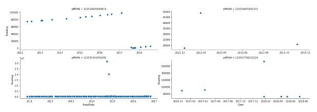
Chart 4-2 - Some examples of MPANs with different anomalous behaviours including spikes and drops in readings, as well as meters resetting.
