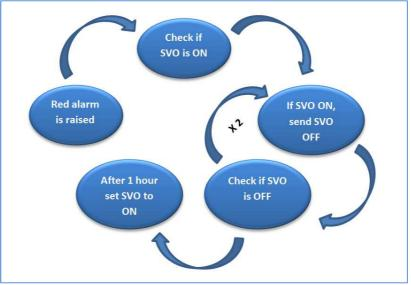
Figure 2-1 Updated Automatic Restoration Procedure
