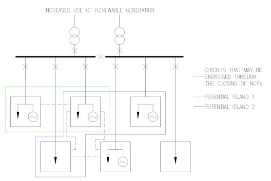
Figure 7-1 Conceptual diagram illustrating islanding for increased use of renewable generation
