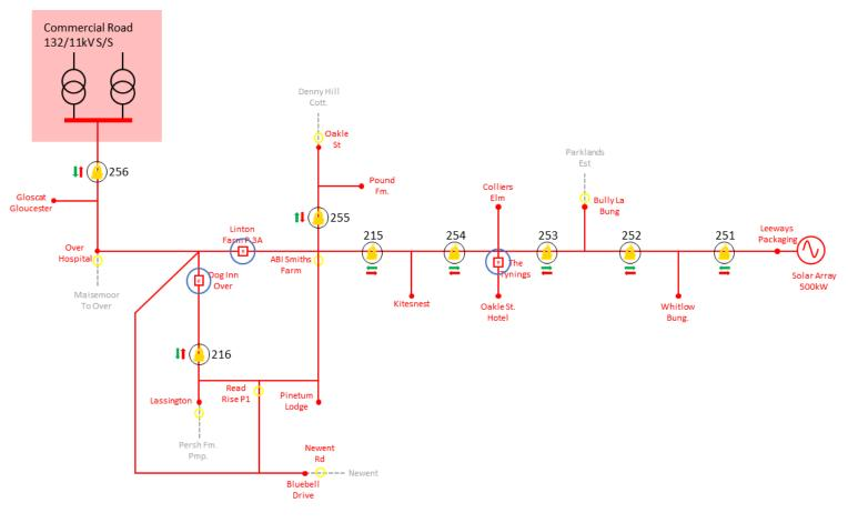
Figure 5-1: The 11kV Distribution Network
