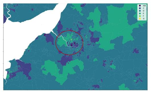
Figure 36: Most common EPC rating amongst households per LSOA. The circled area shows a higher EPC rating, that could be impacting the usage seen in the same area in Figure 35.
