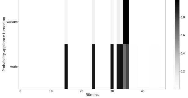
Figure 22: Square plot showing the probability each appliance was turned on for each 30-minute window for the last day the model was run for. The darker the square, the higher the probability.
