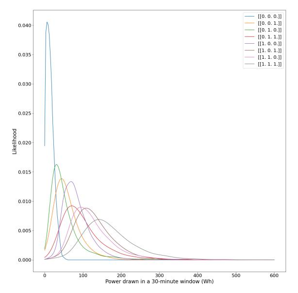
Figure 25: Gaussian kernel-density estimations for the matrix combinations for: kettle, microwave, and toaster, considered for only one 30-minute window.
