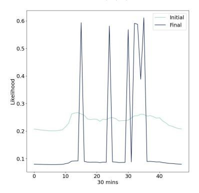
Figure 20: The initial ToD prior for the kettle calculated from the usage statistics alongside the final ToD prior learnt by the model when the same day is repeated. The kettle was turned in on 30-minute windows 15, 24, 30, 32 and 33.
