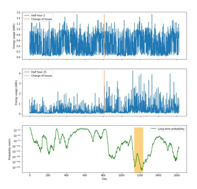
Figure 62: Change detection for increased day time usage (job loss).
