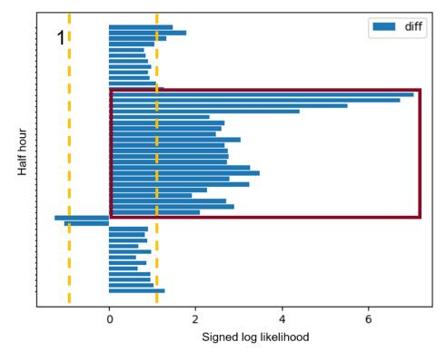
Figure 63: Change fingerprint for increased day time usage (job loss).
