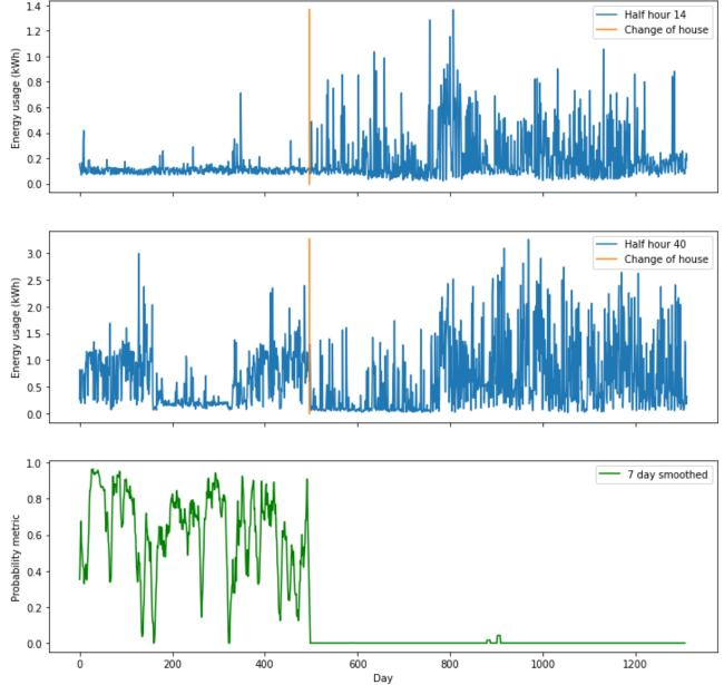
Figure 49: Example short term method output for two houses, with two half hours of underlying data also plotted.
