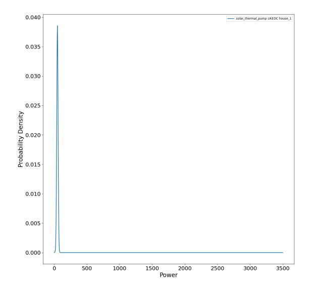
Figure 72: Gaussian kernel-density estimates of the power drawn by each appliance within the heat pump category.
