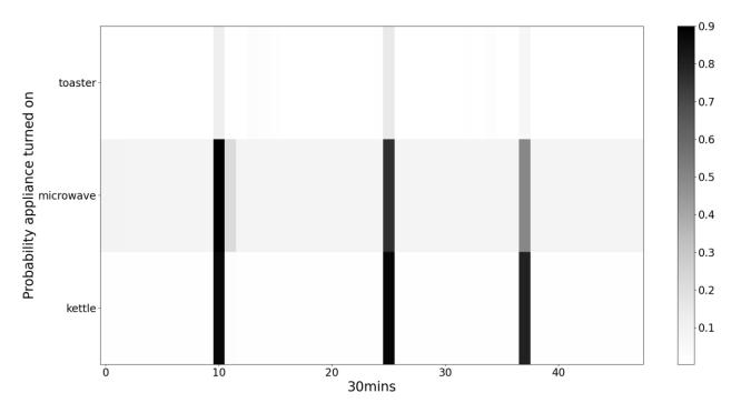
Figure 32: Square plot showing the probability each appliance was turned on for each 30-minute window for the last day the model was run for. *P*<sub>on</sub> is calculated using the matrix likelihoods and the final ToD prior. The darker the square, the higher the probability.
