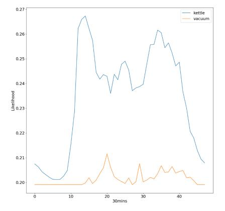
Figure 13: Initial ToD prior for the kettle and vacuum.
