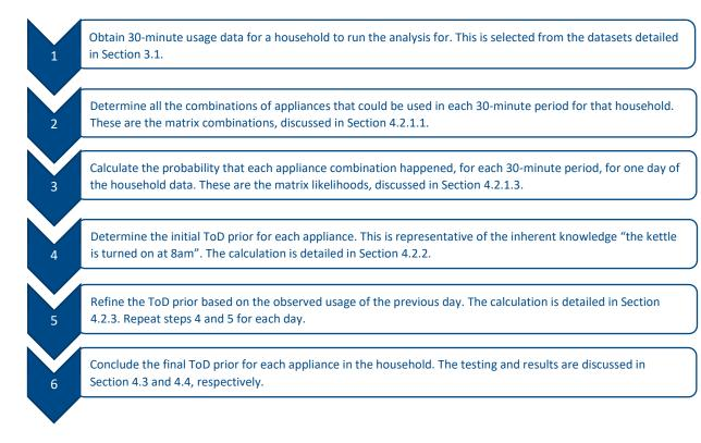
Figure 7: Overview of the appliance disaggregation and prediction method used.
