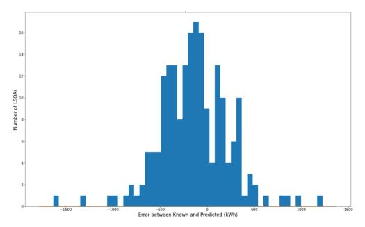
Figure 40: Error distribution between the know average energy usage and the predicted LSOA usage for the testing set of LSOAs.
