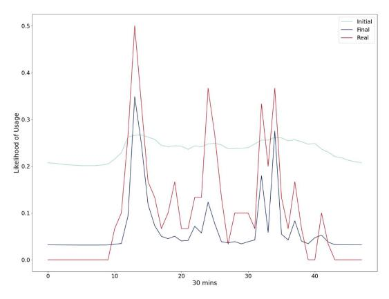
Figure 27: The initial ToD prior for the kettle, calculated from the usage statistics, compared to the final ToD prior for the test household after running the model for 30 days. The real line is the normalised real usage counts.
