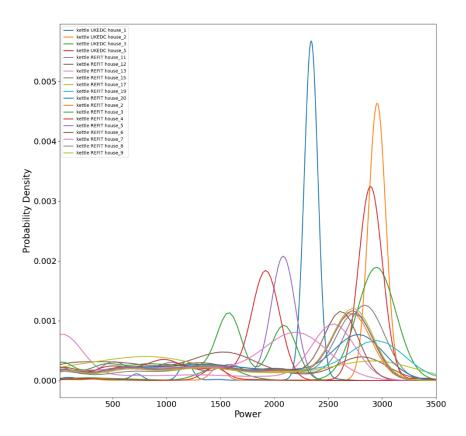
Figure 2: Gaussian kernel-density estimates of the power drawn by each appliance within the kettle category.
