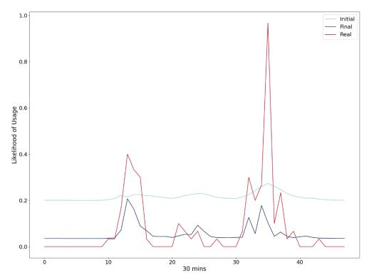
Figure 29: The initial ToD prior for the microwave, calculated from the usage statistics, compared to the final ToD prior for the test household after running the model for 30 days. The real line is the normalised real usage counts.
