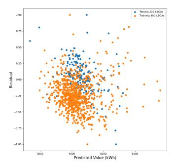
Figure 42: Residual of the known average energy usage per LSOA from the predicted average LSOA against the predicted value for both the training (orange) and the testing (blue) LSOA datasets. The y axis has been normalised using the maximum value of the residual so that the axis varies between 1 and -1.
