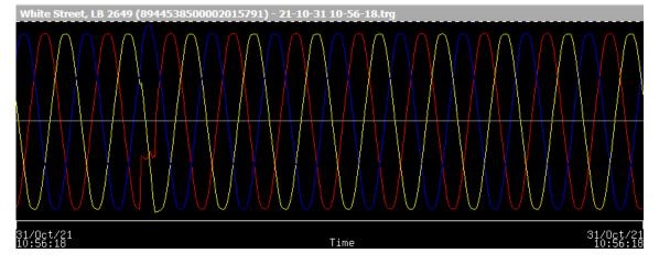
Diagram 10-5: Example of close-up R phase transitory fault showing constant 'arc' voltage drop
