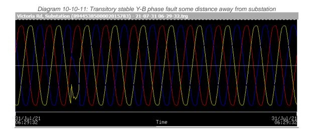
Diagram 10-11Transitory HV system fault on Y phase
