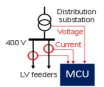
Figure 1 Schematic for the connection of LV monitors for distance to fault assessment
