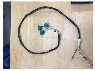
Figure 6: Shielded lead for Clip on current transducers.
