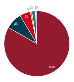
• Gas boiler • Electric (resistive and storage) • Oil boiler • Heat pumps (ASHP, GSHP) • District Heating • Others Source: National Grid ESO, FES (2021). Figure CV.16
