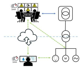
Figure 6-5 - Dispatchable under 1 minute notice requiring API direct to assets with no manual interventions
