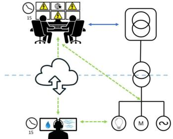
Figure 6-4- Dispatchable with 15 minutes notice requiring API direct to assets with no manual interventions
