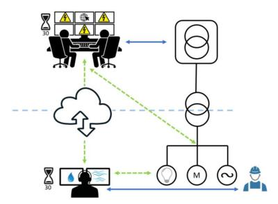
Figure 6-3 – Dispatchable with 30 minutes notice requiring API to site or central control.
