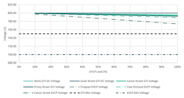
*Figure 12: DC voltages required on the DC side of the GTI to share the load equally between the four GTIs and the EVCP voltages*
