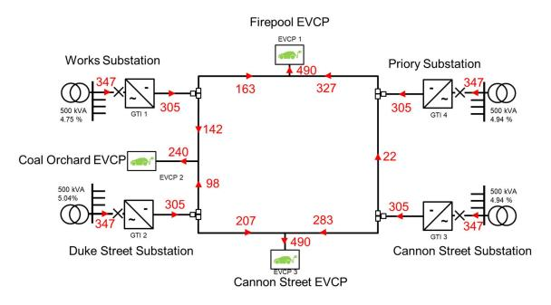
Figure 18. Maximum loading (Intact System) in A
