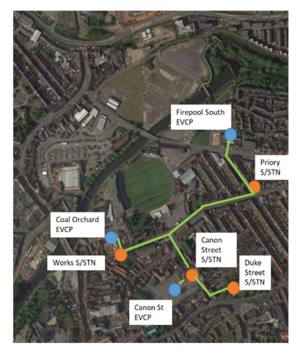
Figure 6: Initial cable route and duct section
