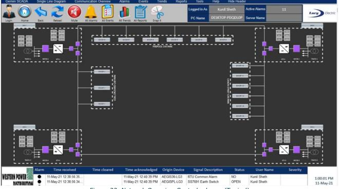
Figure 33. Network Overview Control scheme (Typical)
