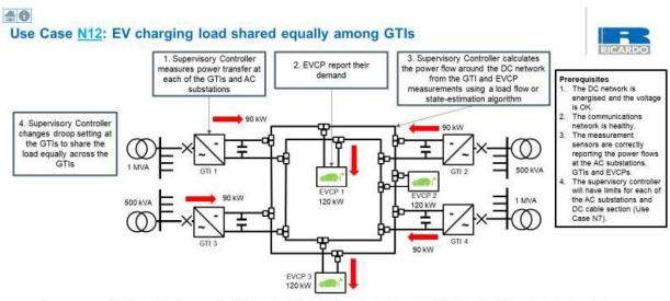
The supervisory controller is provided with an operating limit for each substation. This is expected to be the substation's rating but could be reduced below the rating to demonstrate the supervisory control algorithm.
