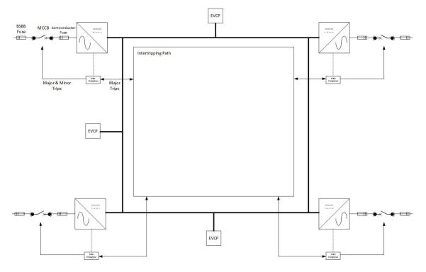
Figure 19: Key line diagram of the overall DC Share System
