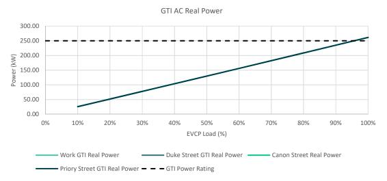
Figure 11: Power flow from the AC side of the GTIs under intact conditions.
