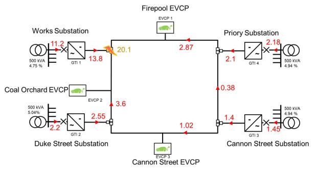
Figure 15. System intact maximum Fault Level Summary in kA
