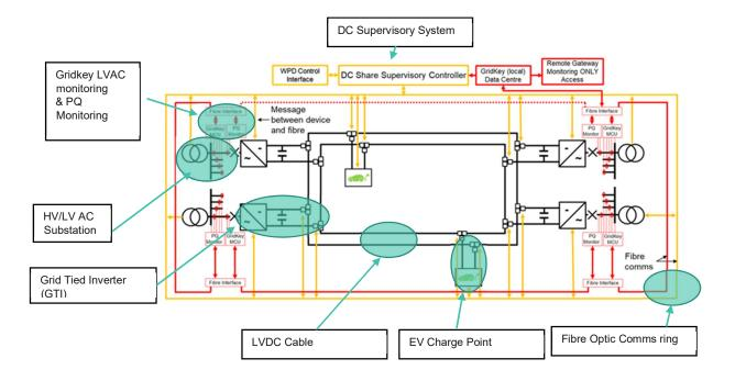
Figure 3: Overview of an LVDC equalisation network
