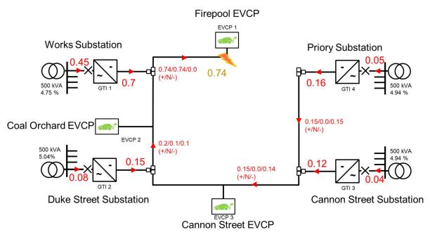
Figure 17. N-1 Scenario minimum Fault Level Summary in A
