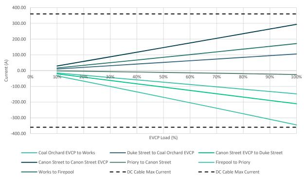
Figure 13: Current flow in the DC cable network
