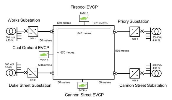
Figure 10: Network schematic of the system that was modelled.
