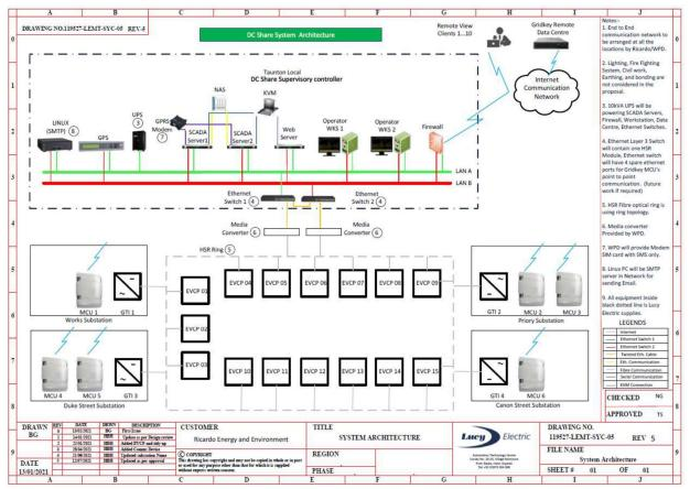
Figure 31. Supervisory Controller system Architecture
