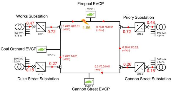
Figure 16. System intact minimum Fault Level Summary in kA
