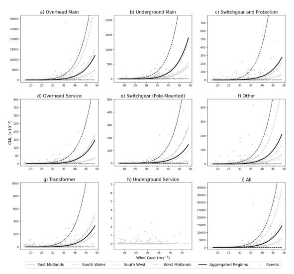
Figure 2 Example fragility curves showing the relationships between wind gust intensity and CML in a windstorm for each asset type.
