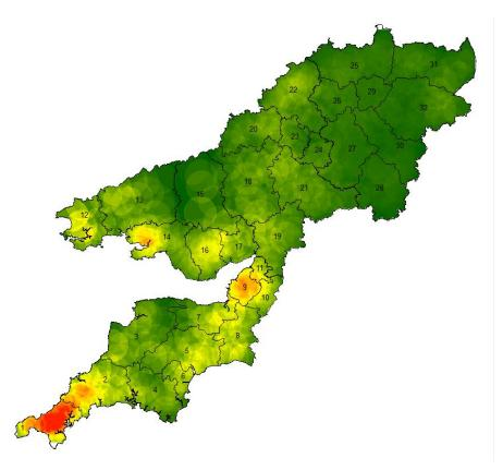
Figure 1 Example heatmap showing number of wind-related faults per primary substation shown on a red/green scale, where red indicates a high number of faults). The highest number of faults recorded is 283.
