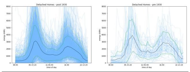
Figure 15 Gas usage for Detached Homes, pre and post 1930 construction by half hour for all days of the heating season. The black line is the mean with green one standard deviation above/below, yellow line is 2 standard deviations.
