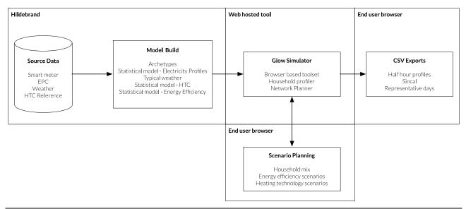
Figure 3 Overall system components with this report detailing the model build and validation from both intermediate results and end user comparison to expected results
