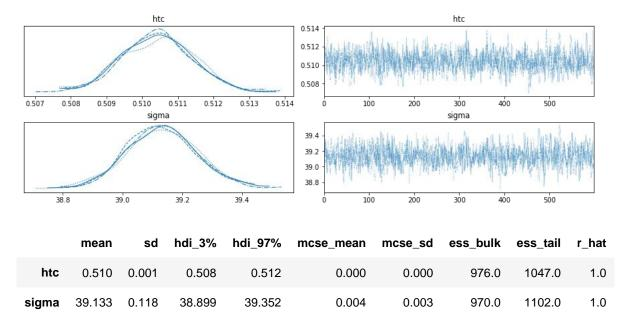
Figure 26 Output from the Bayesian calibration. The four lines show the four independent training runs to fit the model. Variational inference was used, which is more efficient for larger datasets. R-hat = 1 is a strong indicator of fit along with Monte Carlo Standard Error (MCSE) = 0.
