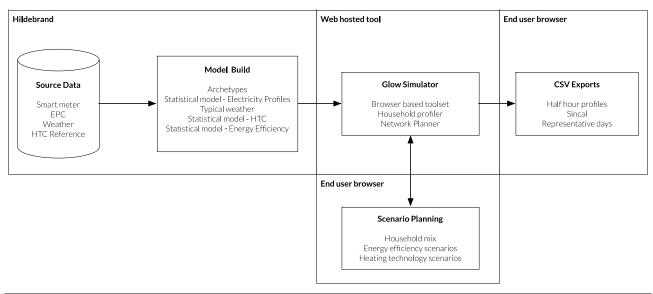
Figure 1 Overall system components with this report detailing the model build and validation from both intermediate results and end user comparison to expected results
