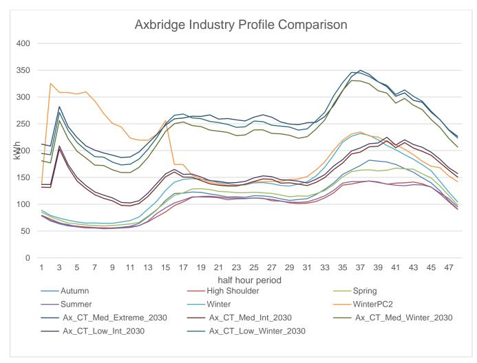
Figure 35 Energy profiles comparing Elexon Profile Class 1 half hour by season for the whole of Axbridge (approximately 252 homes). Winter PC2 applies a Elexon Profile Class 2 (night storage heater) to all of the homes. Scenario labels are the same as above, reduced number to be able to fit on to graph.
