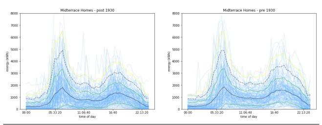
Figure 17 Gas usage for Midterrace Homes, pre and post 1930 construction by half hour for all days of the heating season. The black line is the mean with green one standard deviation above/below, yellow line is 2 standard deviations.
