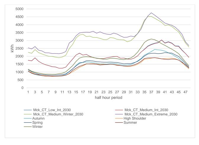
Figure 34 Energy profiles comparing Elexon Profile Class 1 half hour by season for the whole of Mackworth (approximately 3,363 homes). Scenario labels are the same as above, reduced number to be able to fit on to graph.
