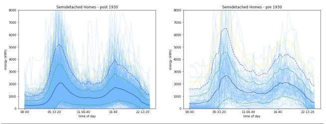
Figure 16 Gas usage for Semi-detached Homes, pre and post 1930 construction by half hour for all days of the heating season. The black line is the mean with green one standard deviation above/below, yellow line is 2 standard deviations.
