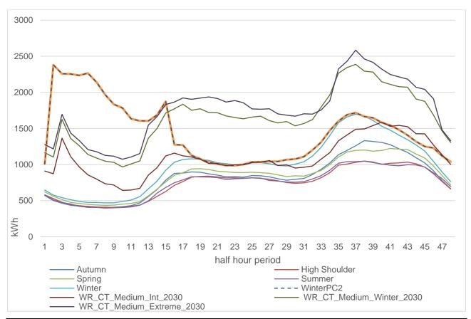
Figure 33 Energy profiles comparing Elexon Profile Class 1 half hour for the whole of WithycombeRaleigh (approximately 1,843 homes). Winter PC2 applies a Elexon Profile Class 2 (night storage heater) to all of the homes. Scenario labels are the same as above, reduced number to be able to fit on to graph.
