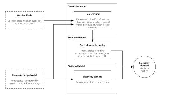
Figure 4 Details of the model elements as they are used to generate data; the data sources and model parameters are in the code running on an end user's browser
