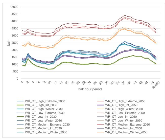
Figure 30 Energy profiles for heating simulated for the whole of WithycombeRaleigh (approximately 1,843 homes) and takeup of heat pumps using percentage offsets to the HTC random variable, results are in the expected order
