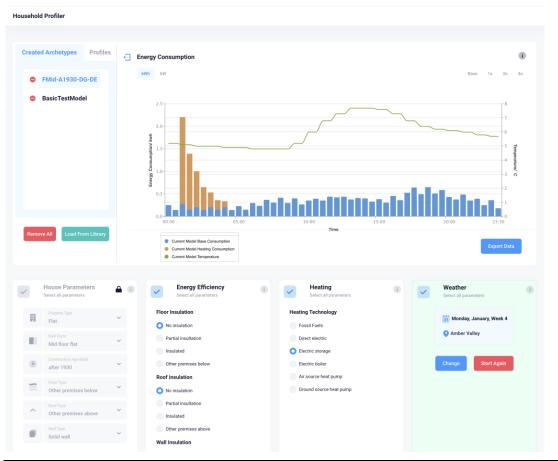
Figure 42 Result of applying electric storage as a heating type to a Mid-floor flat; this is to illustrate the charging decay function and how it is applied
