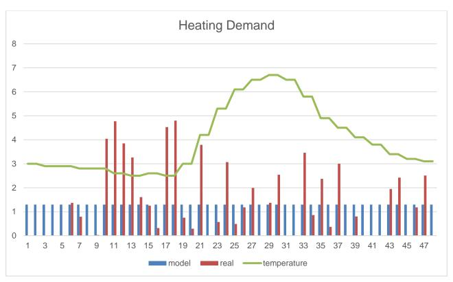
Figure 47 Model (blue) energy for heat and real gas usage (red) for a Thursday 27 Junary 2022, both in kWh units. Temperature is overlayed in green. A heat pump model is used for the simulated data.
