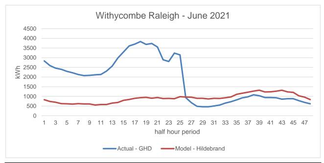
Figure 52 Large overnight load in June 2021 for Withycombe Raleigh which is an anomaly
