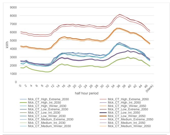
Figure 31 Energy profiles for heating simulated for the whole of Mackworth (approximately 3,363 homes) and takeup of heat pumps using percentage offsets to the HTC random variable, results are in the expected order
