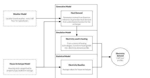
Figure 2 Details of the model elements as they are used to generate data; the data sources and model parameters are in the code running on an end user's browser
