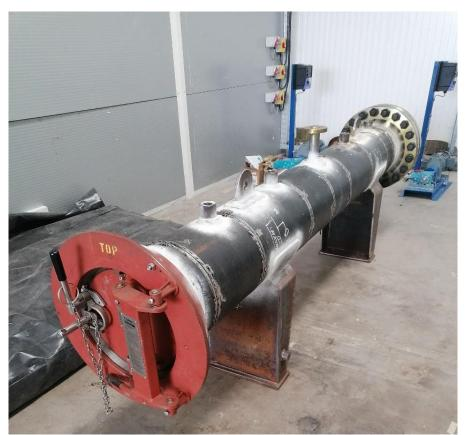
Figure 8 Extraction vessel showing the Bandlock 2 quick opening enclosure and prior to the application of heating tape, insulation and aluminium shell
