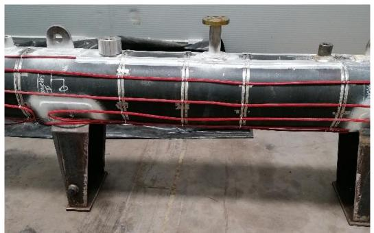
Figure 9 Extraction vessel with heat tracing (red) applied
