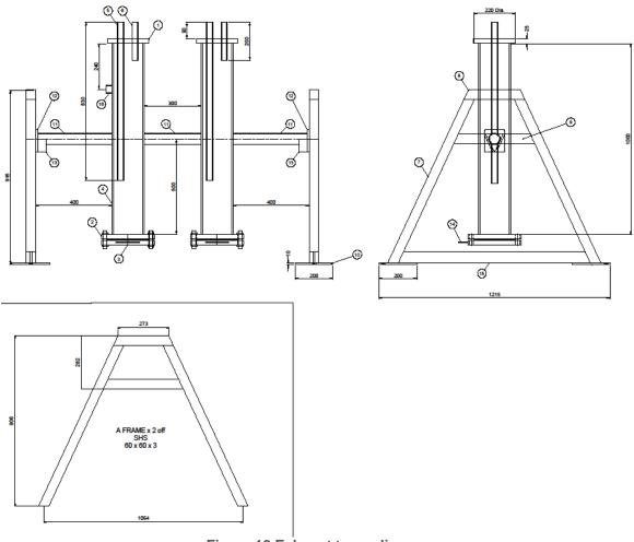
Figure 18 Exhaust traps diagram
