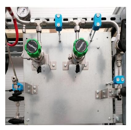
Figure 13 Swagelok high pressure back pressure regulators
