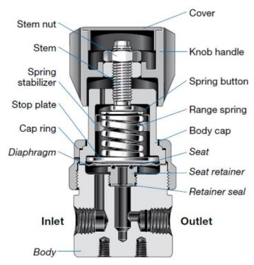
Figure 12 Swagelok spring loaded back pressure regulator
