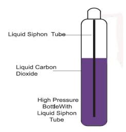
Figure 1 Liquid carbon dioxide cylinder delivery system
