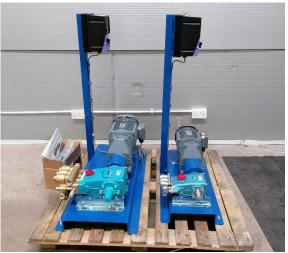
Figure 5 Liquid carbon dioxide pumps
