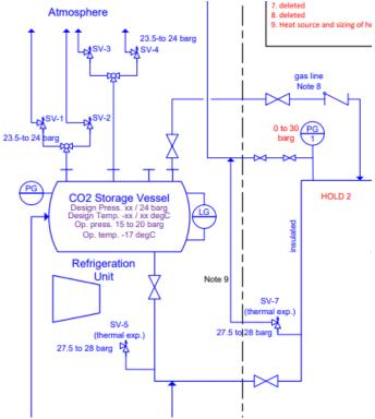
Figure 3 Storage tank safety pressure relief diagram
