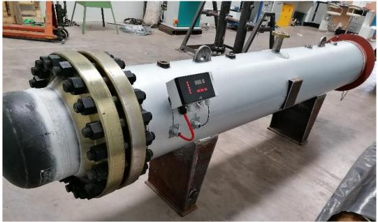
Figure 10 Completed extraction vessel
