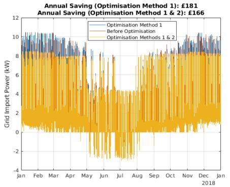
Figure 3.11 - Optimisation Methods 1 & 2: Delayed EV charging & modified heat demand grid import profile
