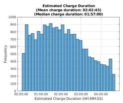
Figure 2.5 - Distribution of estimated charge duration for 33kWh, 7kW vehicles during the Electric Nation trial
