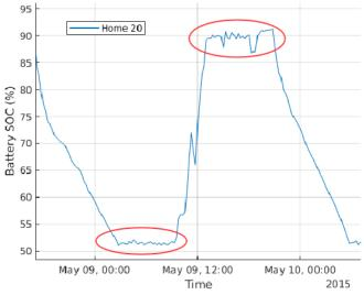
Figure 2.14 - Battery SOC oscillations at the SOC thresholds for Home 20 on 9th May 2015
