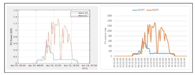
Figure 2.10 - Calculated PV power against actual PV power for homes 15 and 16 on 15th April 2015
