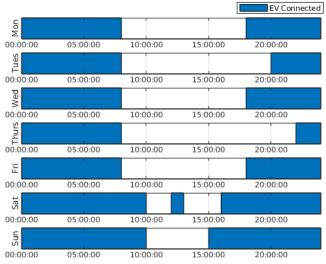
Figure 3.1 - Commuter EV usage pattern used in the modelling, showing when the EV is connected to the chargepoint.
