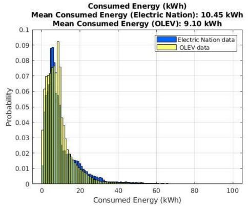
Figure A1.3 - Energy consumption distribution comparison for Electric Nation and OLEV data sets
