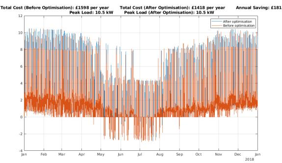
Figure 3.7 - Optimisation Method 1: Delayed EV charging grid import profile
