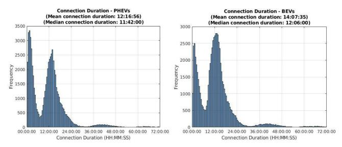
Figure 2.2 - Distribution of connection durations during the Electric Nation trial (PHEV/BEV Breakdown)
