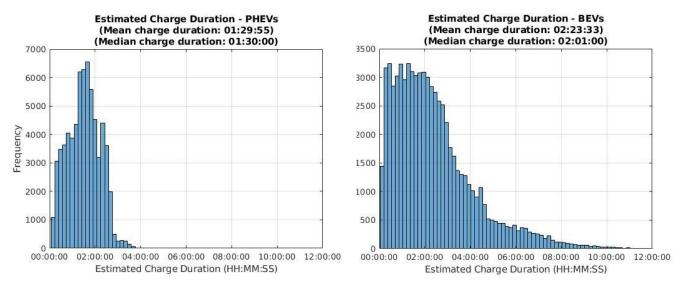
Figure 2.4 - Distribution of estimated charge durations during the Electric Nation trial (PHEV/BEV Breakdown)
