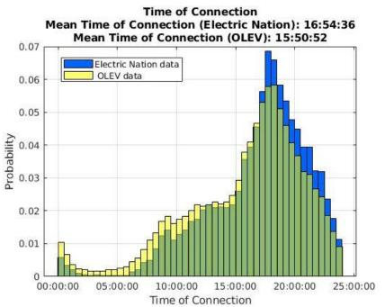
Figure A1.2 - Time of Connection distribution comparison for Electric Nation and OLEV data sets
