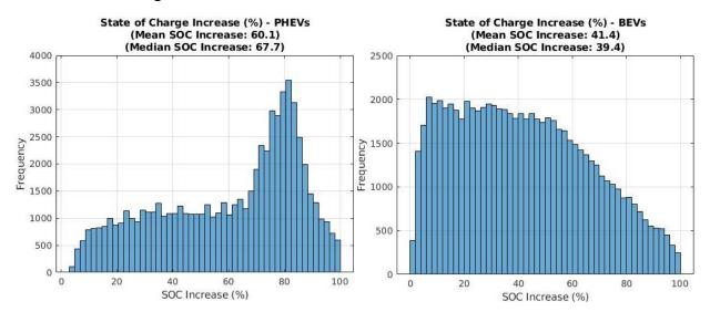
Figure 2.10 - Distribution of SOC increase during the Electric Nation trial (PHEV/BEV Breakdown)
