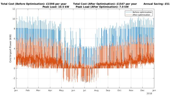
Figure 3.14 - Constrained EV charging grid import profile, with charging constrained to half power (3.5kW)
