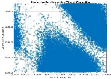
Figure 2.8 - Connection duration against time of connection during the Electric Nation trial
