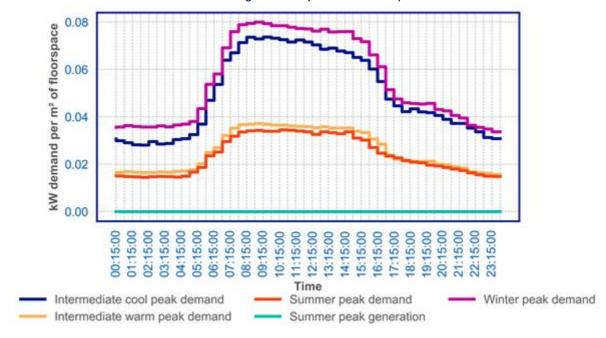
Figure 76: B2 non domestic resistive electric heating demand per m<sup>2</sup> of floorspace
