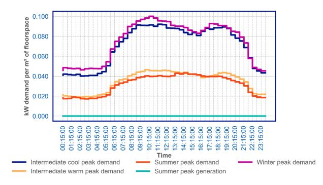
Figure 86: D2 non domestic resistive electric heating demand per m<sup>2</sup> of floorspace
