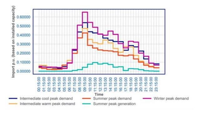
Figure 52: En-route / local charging stations, Car parks and Destination unabated kW per kW installed capacity representative day charging profile
