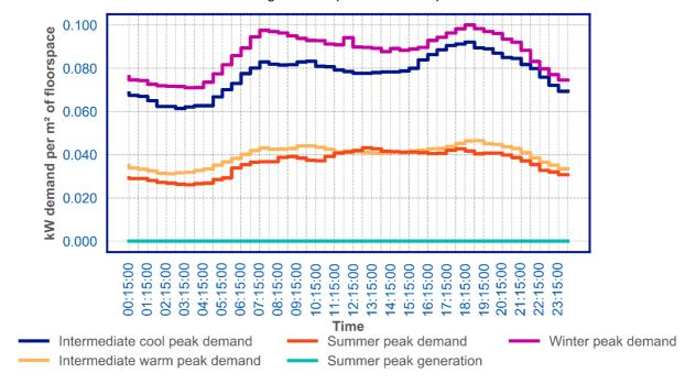
Figure 80: C1 non domestic resistive electric heating demand per m<sup>2</sup> of floorspace
