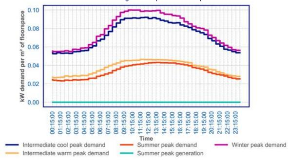
Figure 70: A1/A2 non domestic resistive electric heating demand per m<sup>2</sup> of floorspace
