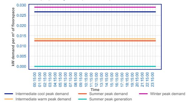
Figure 83: D1 non domestic heat pump heating demand per m<sup>2</sup> of floorspace
