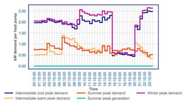
Figure 62: Non-hybrid ground source heat pump with thermal storage profiles in baseline year
