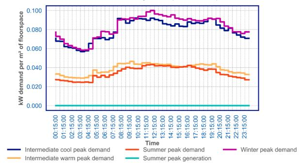
Figure 88: Sui Generis non domestic resistive electric heating demand per m2 of floorspace
