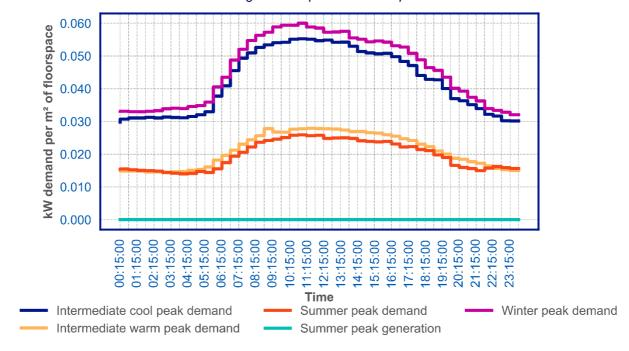
Figure 82: C2 non domestic resistive electric heating demand per m<sup>2</sup> of floorspace
