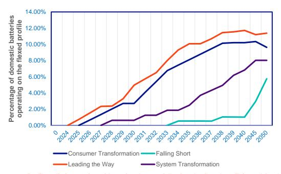
Figure 22: Profile split (proportion of batteries that are following the flexed profile) used for domestic batteries in each DFES scenario.
