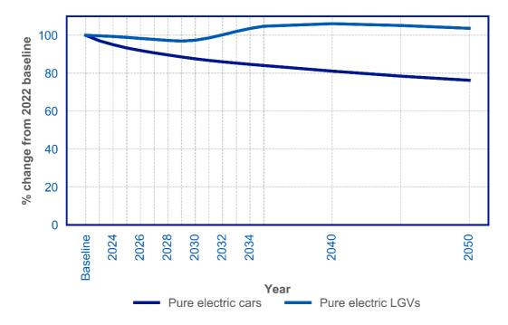
Figure 54: Car and LGV efficiency improvement assumptions taken from DfT TAG model
