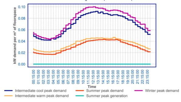
Figure 72: A3/A4/A5 non domestic resistive electric heating demand per m² of floorspace
