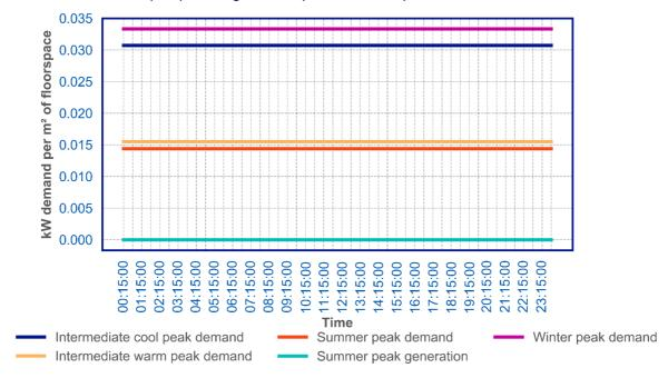
Figure 85: D2 non domestic heat pump heating demand per m<sup>2</sup> of floorspace
