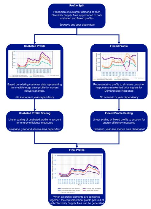
Figure 4: Representation of how customer behavioural changes are applied to the profiles for DFES analysis
