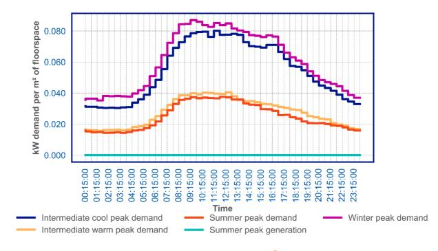
Figure 84: D1 non domestic resistive electric heating demand per m<sup>2</sup> of floorspace
