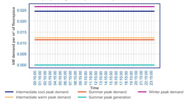
Figure 77: B8 non domestic heat pump heating demand per m<sup>2</sup> of floorspace
