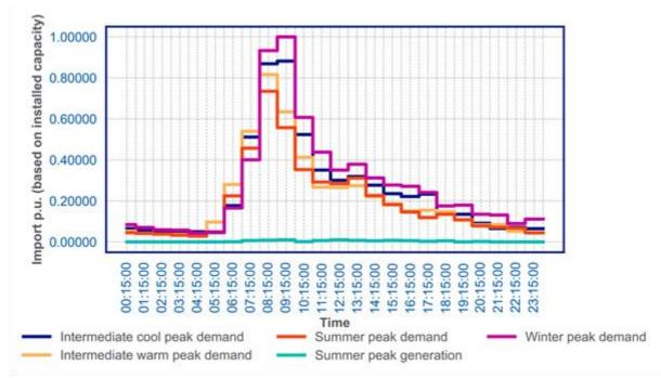
Figure 51: Workplace and fleet/depot unabated kW per kW installed capacity representative day charging profile
