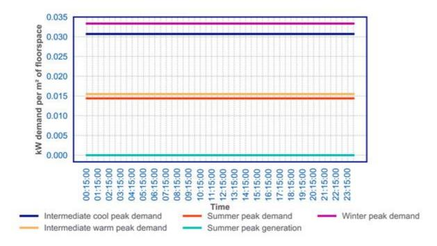
Figure 71: A3/A4/A5 non domestic heat pump heating demand per m<sup>2</sup> of floorspace
