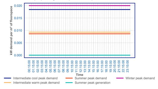
Figure 81: C2 non domestic heat pump heating demand per m² of floorspace
