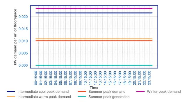
Figure 73: B1 non domestic heat pump heating demand per m<sup>2</sup> of floorspace
