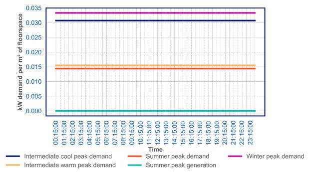
Figure 79: C1 non domestic heat pump heating demand per m<sup>2</sup> of floorspace
