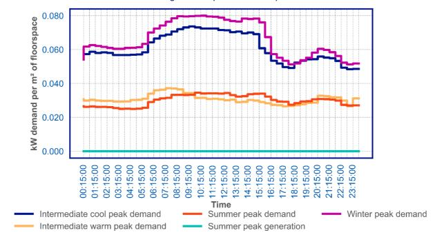
Figure 78: B8 non domestic resistive electric heating demand per m<sup>2</sup> of floorspace
