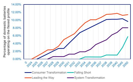
Figure 38: Profile split (proportion of batteries that are following the flexed profile) used for domestic batteries in each DFES scenario.
