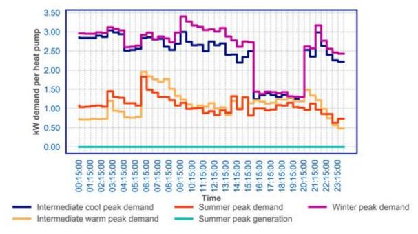
Figure 61: Non-hybrid air source heat pump with thermal storage profiles in baseline year
