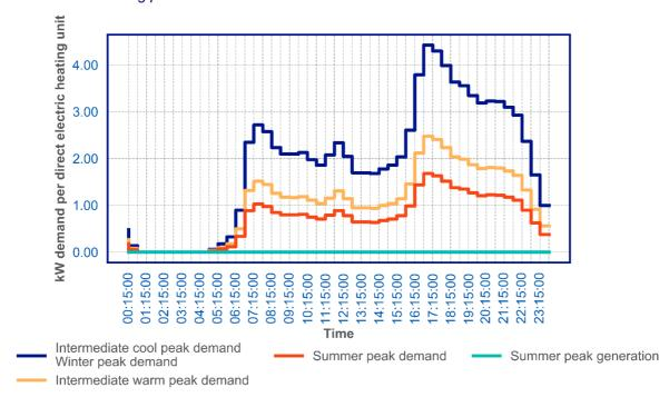
Figure 56: Direct Electric heating profile per installation in baseline year
