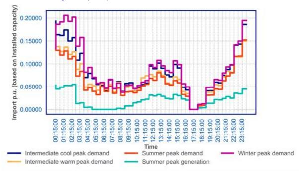
Figure 50: Residential managed charging (flexed) kW per kW installed capacity representative day charging profile
