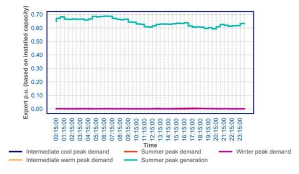
Figure 11: Representative less than 1MW onshore wind profiles for customers in the South West licence area
