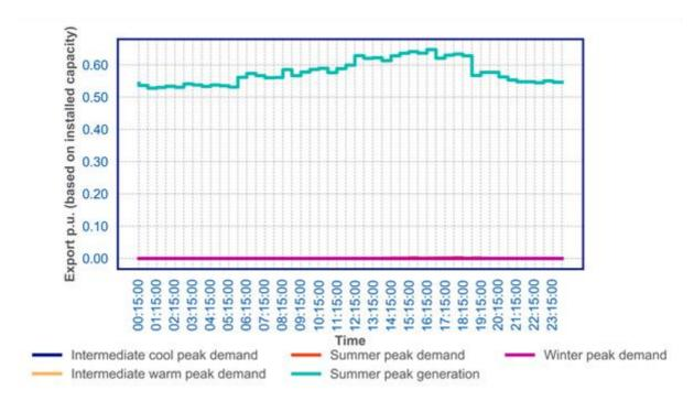
Figure 10: Representative greater than or equal to 1MW onshore wind profiles for customers in the South West licence area
