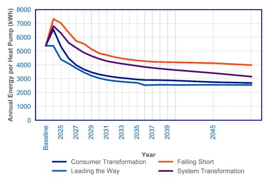
Figure 66: Yearly energy requirement per non-hybrid air source heat pump
