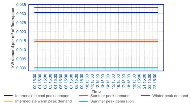
Figure 87: Sui Generis non domestic heat pump heating demand per m<sup>2</sup> of floorspace
