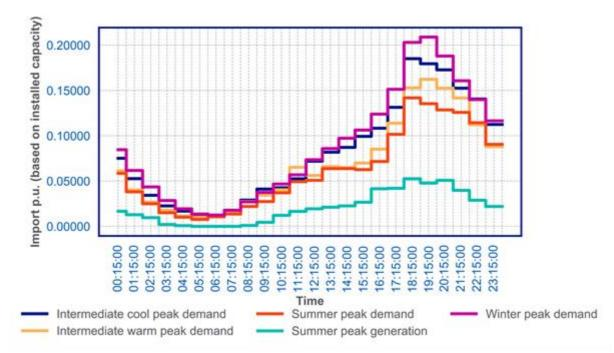
Figure 49: Residential unabated kW per kW installed capacity representative day charging profile
