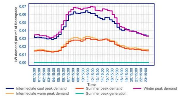
Figure 74: B1 non domestic resistive electric heating demand per m<sup>2</sup> of floorspace
