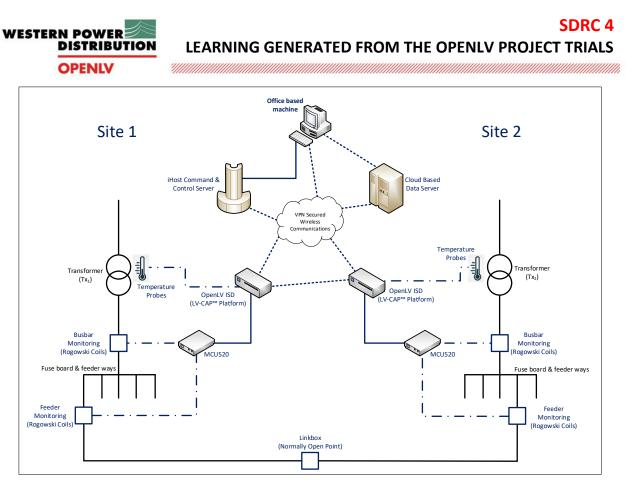
Figure 4: LV network arrangement and LV-CAP deployment
