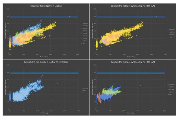
Figure 27: Calculated Hot Spot vs % Loading (Tx Groupings)
