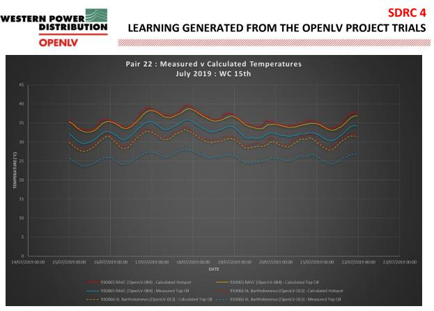
Figure 8: Pair 22 - Measured vs Calculated Temperatures
