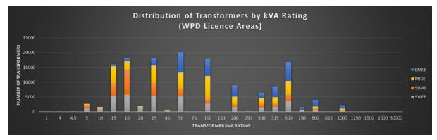
Figure 25: Distribution of Transformers by kVA Rating
