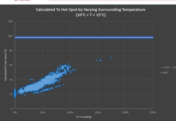
Figure 34: Calculated Tx Hot Spot by Surrounding Temperature (10°C < T < 15°C)
