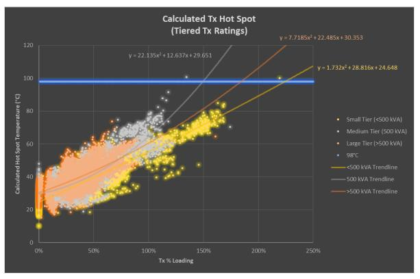
Figure 28: Forecasting Tx Hot Spot Temperatures
