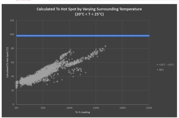
Figure 32: Calculated Tx Hot Spot by Surrounding Temperature (20°C < T < 25°C)
