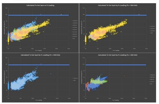
Figure 16: Calculated Hot Spot vs % Loading (Tx Groupings)
