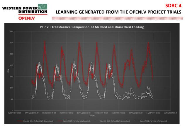
Figure 21: Pair 2 – Transformer Comparison – Meshed & Unmeshed Loading
