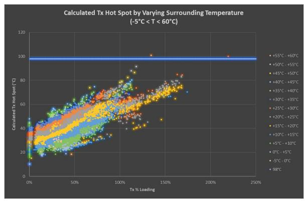
Figure 29: Calculated Tx Hot Spot by Surrounding Temperature (-5°C < T < 60°C)
