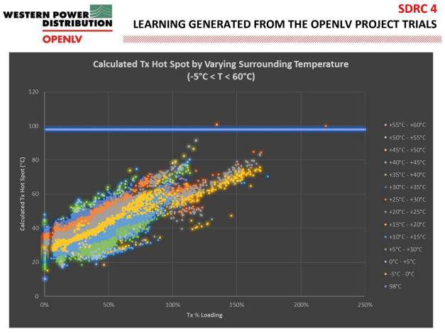
Figure 18: Calculated Tx Hot Spot in relation to surrounding temperature
