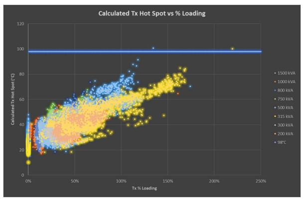
Figure 26: Calculated Hot Spot vs % Loading
