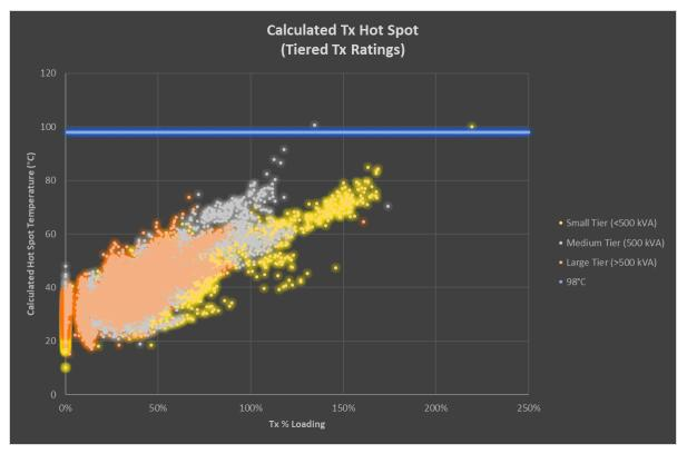
Figure 22: Calculated Tx Hot Spots by % Loading
