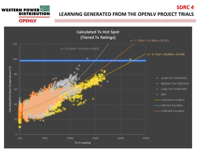
Figure 17: Forecasting Tx Hot Spot Temperatures
