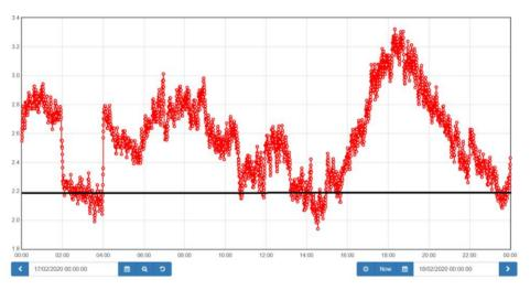
Fig 2. Plot showing subsea cable loading over an average day (red) and where a +2.2MW limit would have triggered system operation.
