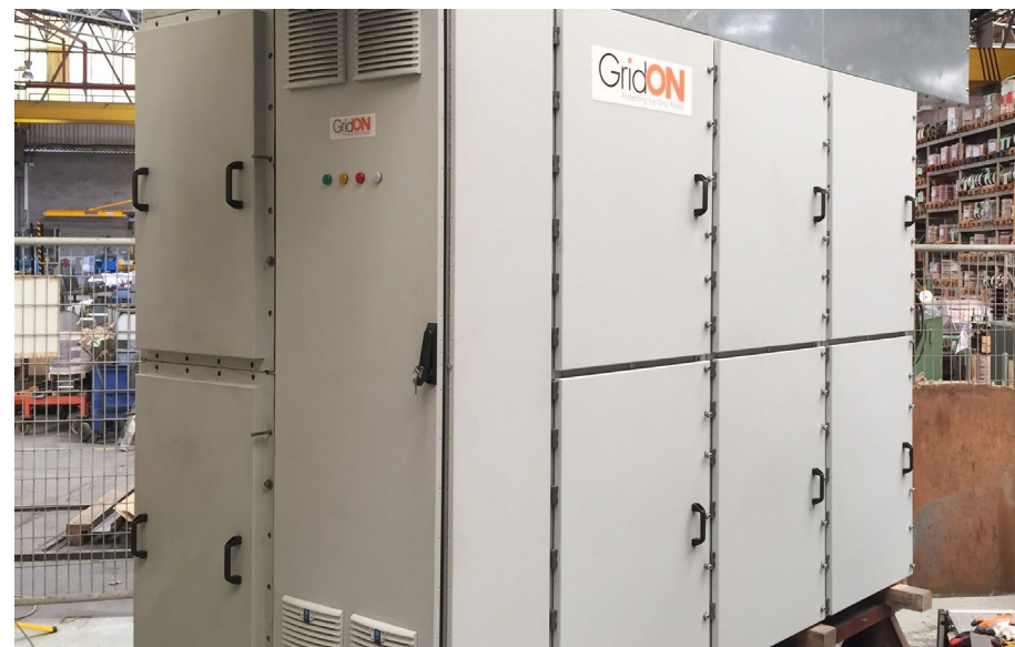
FCLi device being tested
