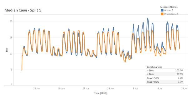
Figure 50. Load customer – SCADA – Jaguar Land Rover – 1 day
