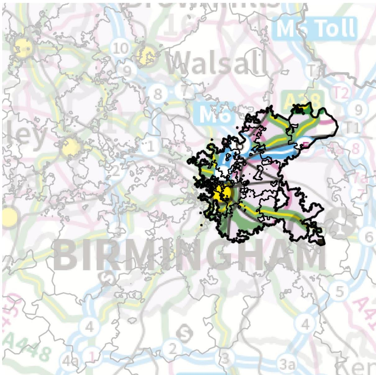
Figure 35: Area supplied by Nechells GSP
