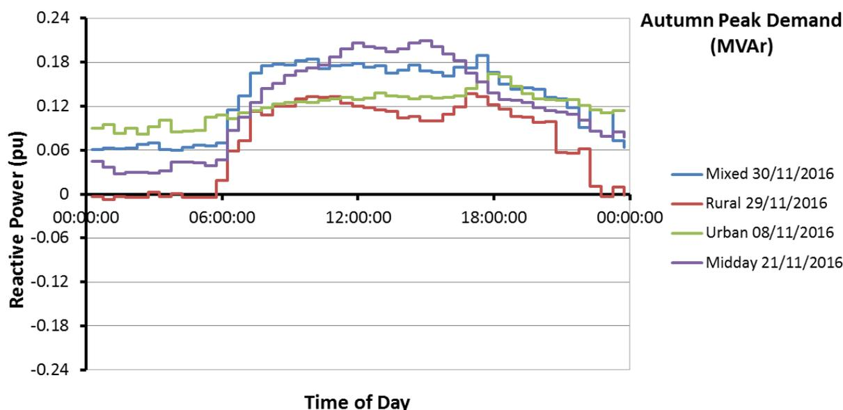
Figure 15: Reactive power underlying demand profiles for the Autumn Peak Demand day, normalised over the peak real power annual demand (note: reactive power scale is not the same as the active power scale)
