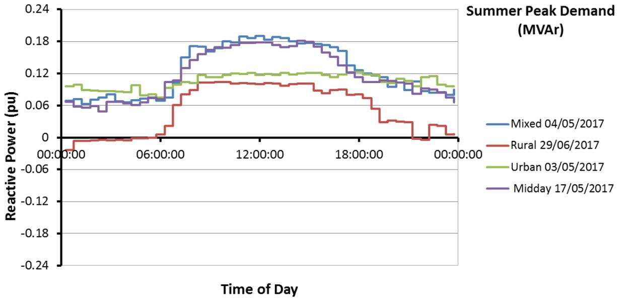
Figure 11: Reactive power underlying demand profiles for the Summer Peak Demand day, normalised over the peak real power annual demand (note: reactive power scale is not the same as the active power scale)
