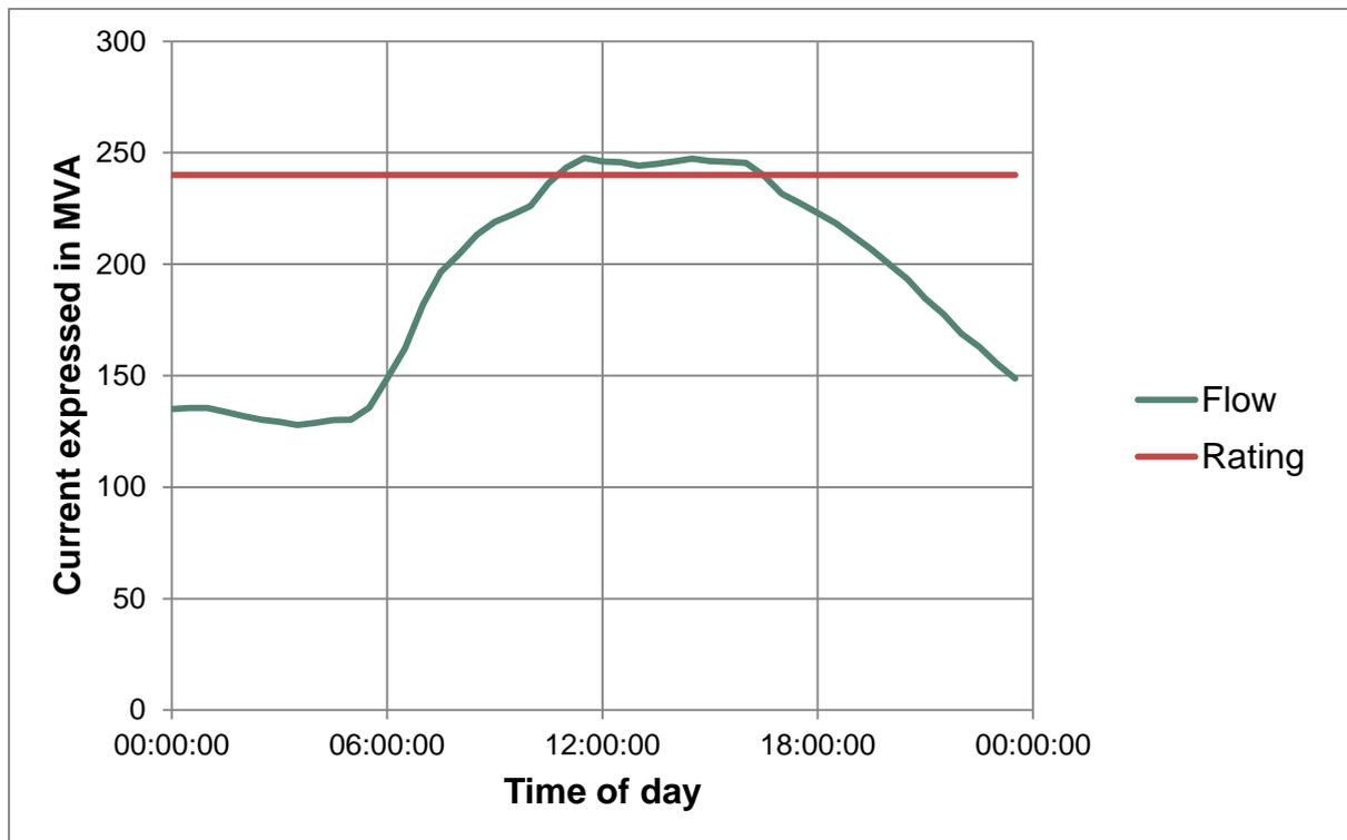
**Figure 36: Graph of Nechells SGT1 loading (Consumer Power 2020, Autumn Peak Demand day, during outage of Nechells SGT3)**
