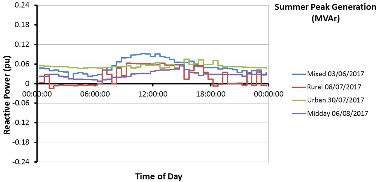
Figure 13: Reactive power underlying demand profiles for the Summer Peak Generation day, normalised over the peak real power annual demand (note: reactive power scale is not the same as the active power scale)
