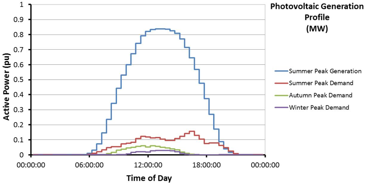
Figure 19: Normalised PV generation profile for each representative day
