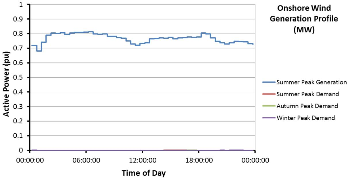
Figure 23: Normalised Onshore Wind generation profile used for each representative day. Note that due to the scale, the profiles for the demand days are near-zero
