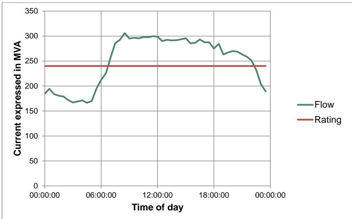
Figure 45: Graph of Shrewsbury SGT3 loading (Gone Green 2020, Summer Peak Demand day, during outage of both 132kV circuits from Ironbridge)
