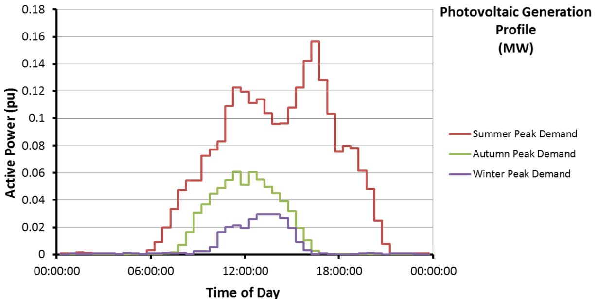
Figure 20: Detailed view of normalised PV generation profiles used for the Summer Peak, Autumn Peak and Winter Peak demand representative days
