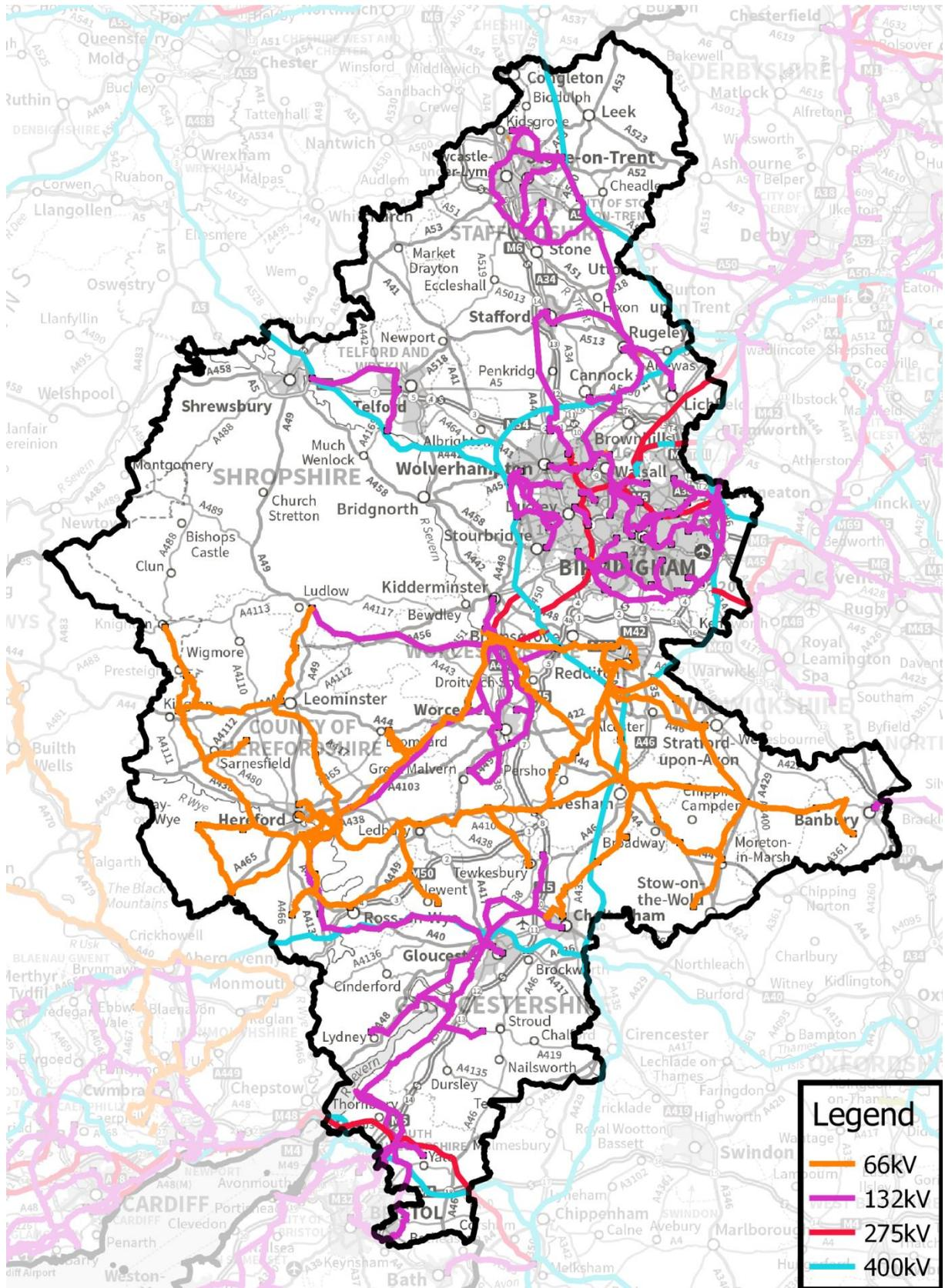
Figure 1: Network in West Midlands showing 400kV, 275kV, 132kV and 66kV networks
