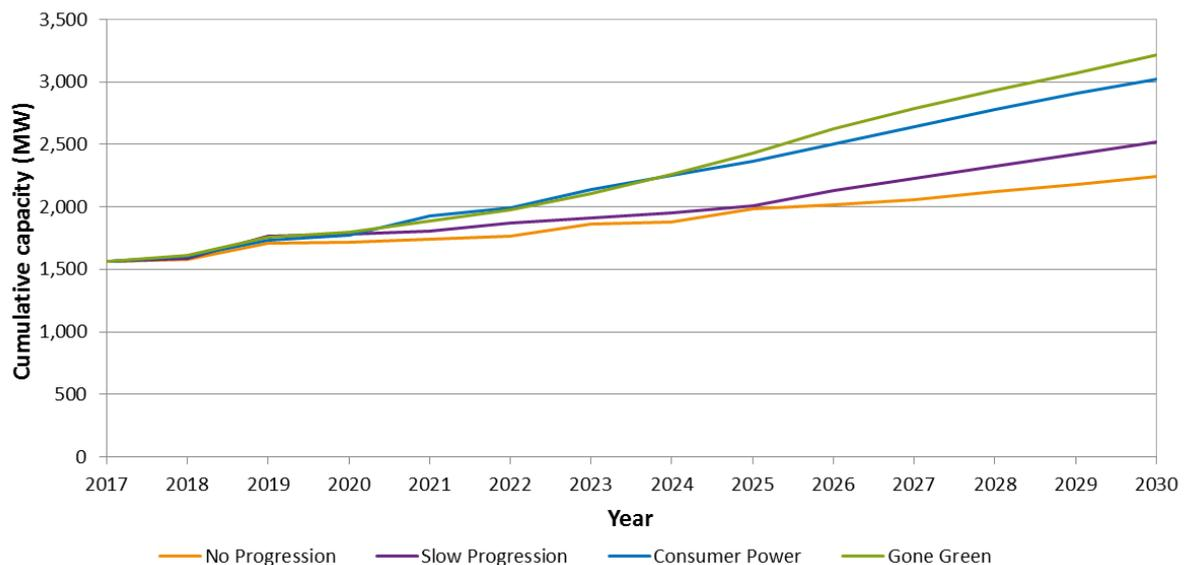
**Figure 6: Total Distributed Generation capacity growth in WPD West Midlands licence area from 2017 to 2030 under each scenario**
