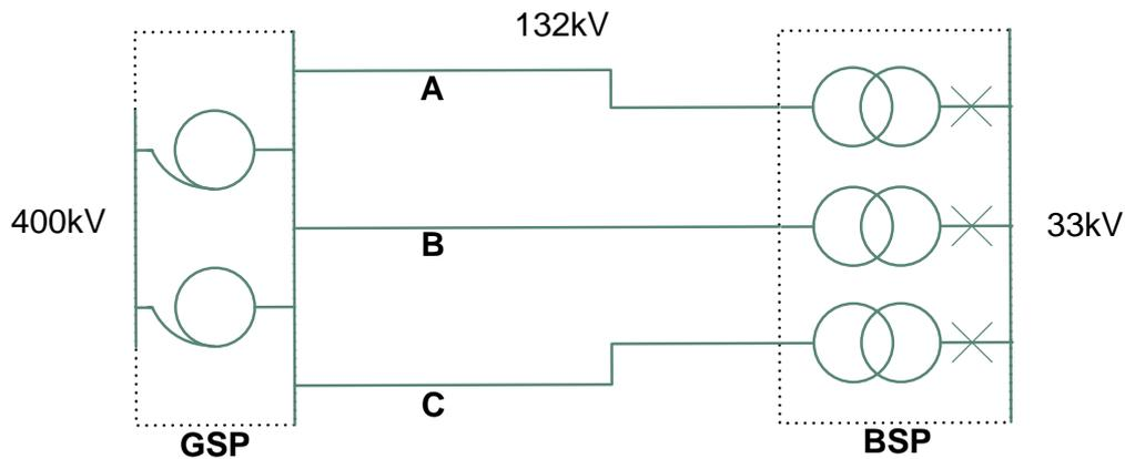
**Figure 25: Three-circuit group example**
