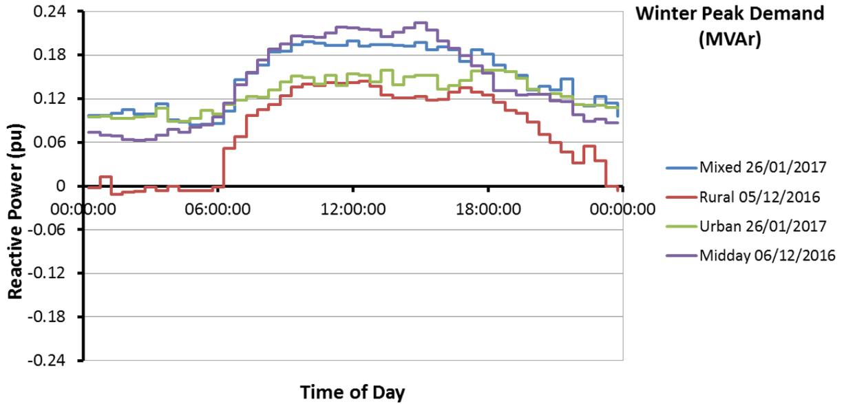
Figure 9: Reactive power underlying demand profiles for the Winter Peak Demand day, normalised over the peak real power annual demand (note: reactive power scale is not the same as the active power scale)
