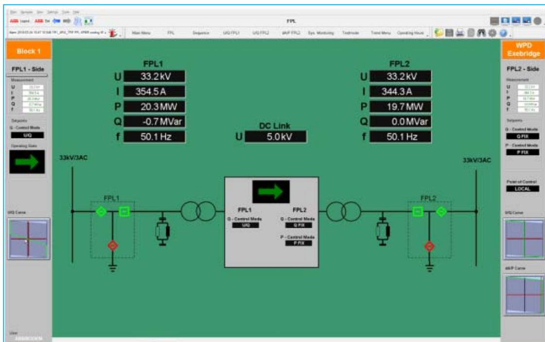
Figure 5-11: Screen shot of FPL HMI during Hot Commissioning
