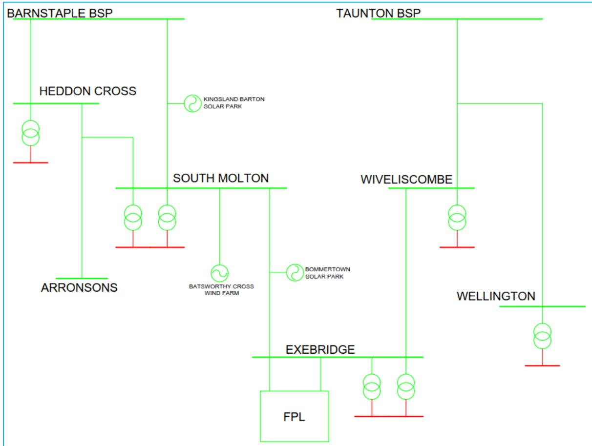
Figure 2-22: Overview of 33kV Network Modelled within the FPL CM
