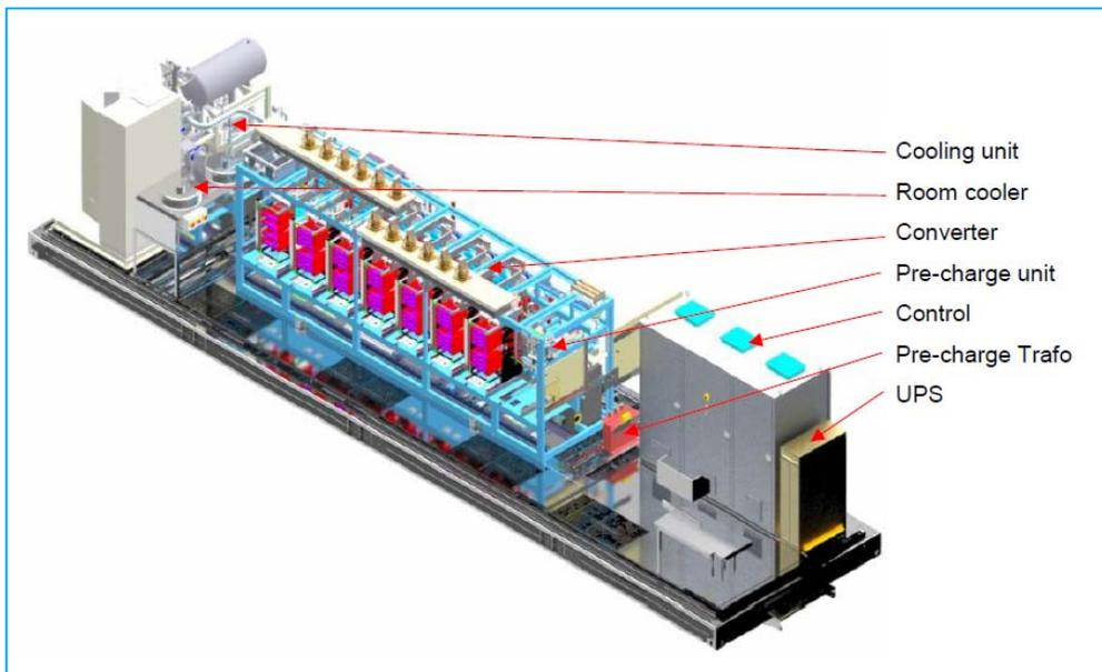
Figure 2-6: Internal view of FPL container
