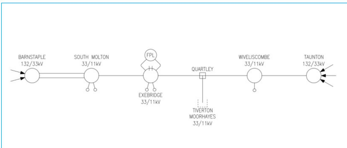
Figure 1-4: High Level Single Line Diagram of 33kV Network between Barnstaple and Taunton BSPs
