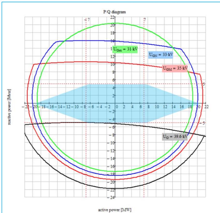
Figure 2-3: ABB FPL Device Operating Window
