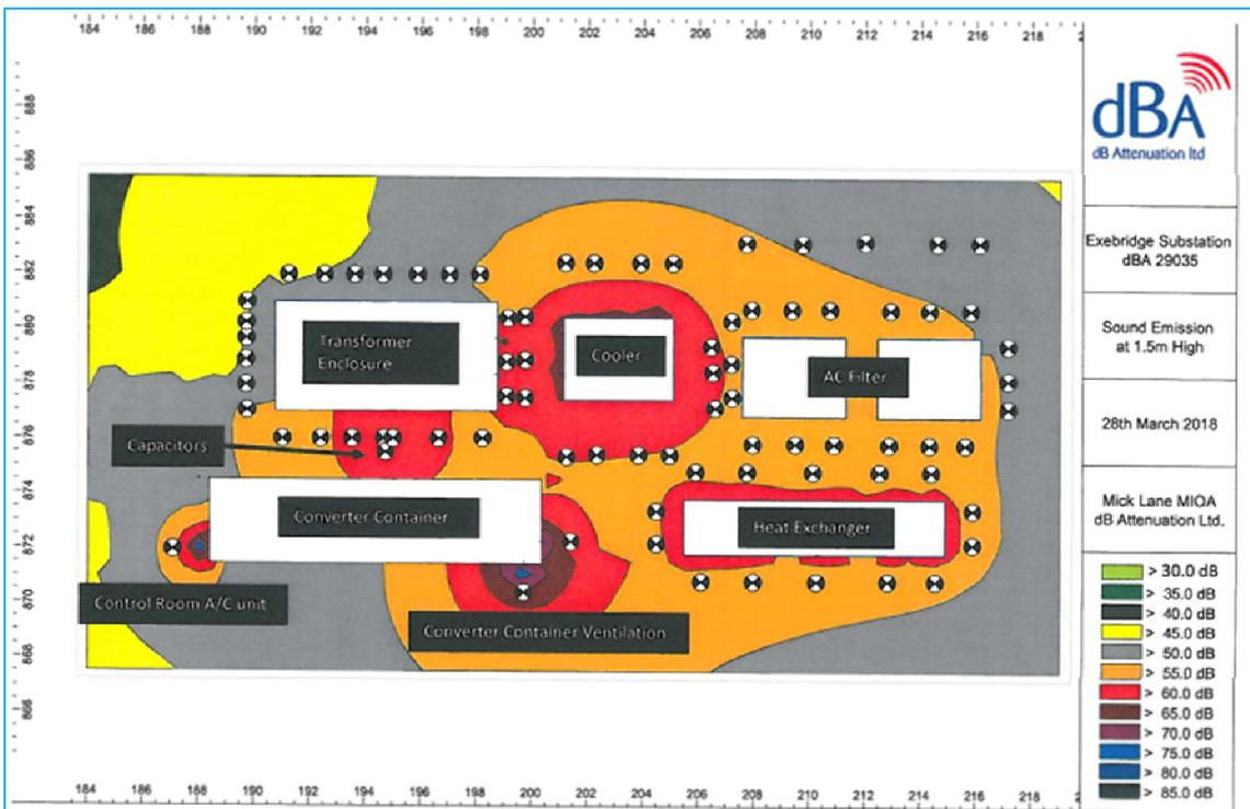
Figure 5-16: Sound Emissions with FPL Operating at Maximum Power Output
