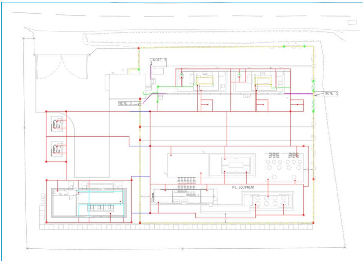
Figure 3-21: Earthing Design for Exebridge
