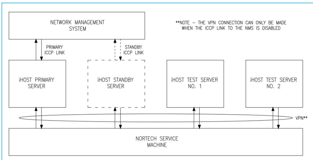
Figure 2-19: FPL Control Module Architecture Overview
