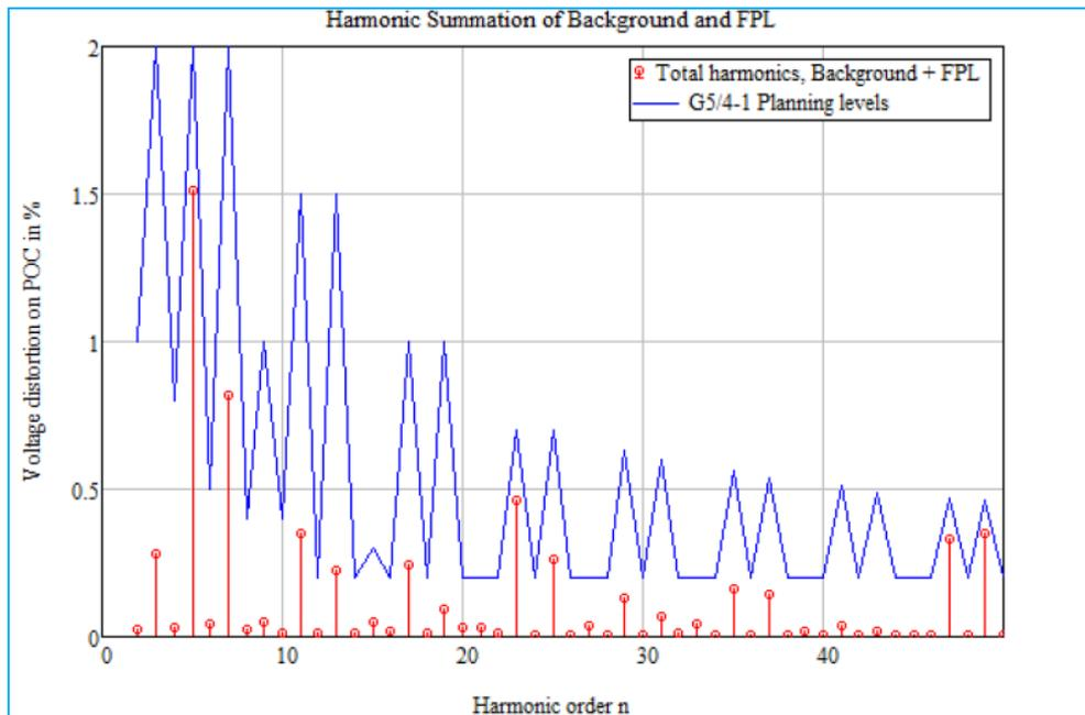
Figure 5-17: Harmonic Survey Results post FPL installation
