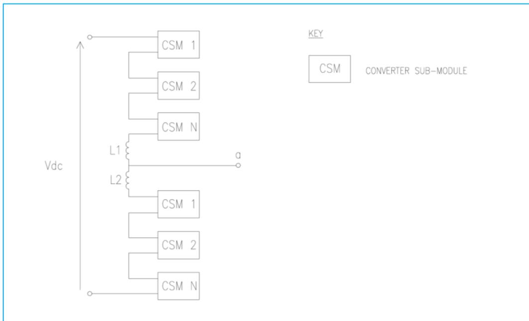
**Figure 8-5: Multilevel converter architecture**
