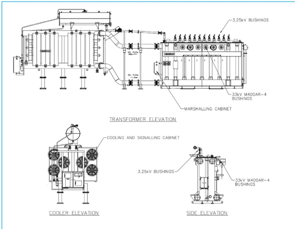
Figure 2-12: FPL transformer elevations
