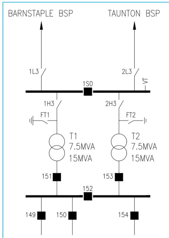
Figure 3-2: Original Single Line Diagram for Exebridge Substation
