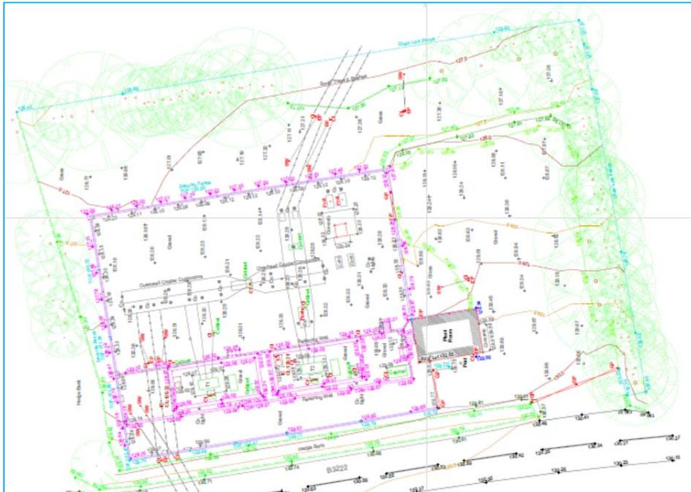
Figure 3-4: Topographical Survey of Exebridge Substation
