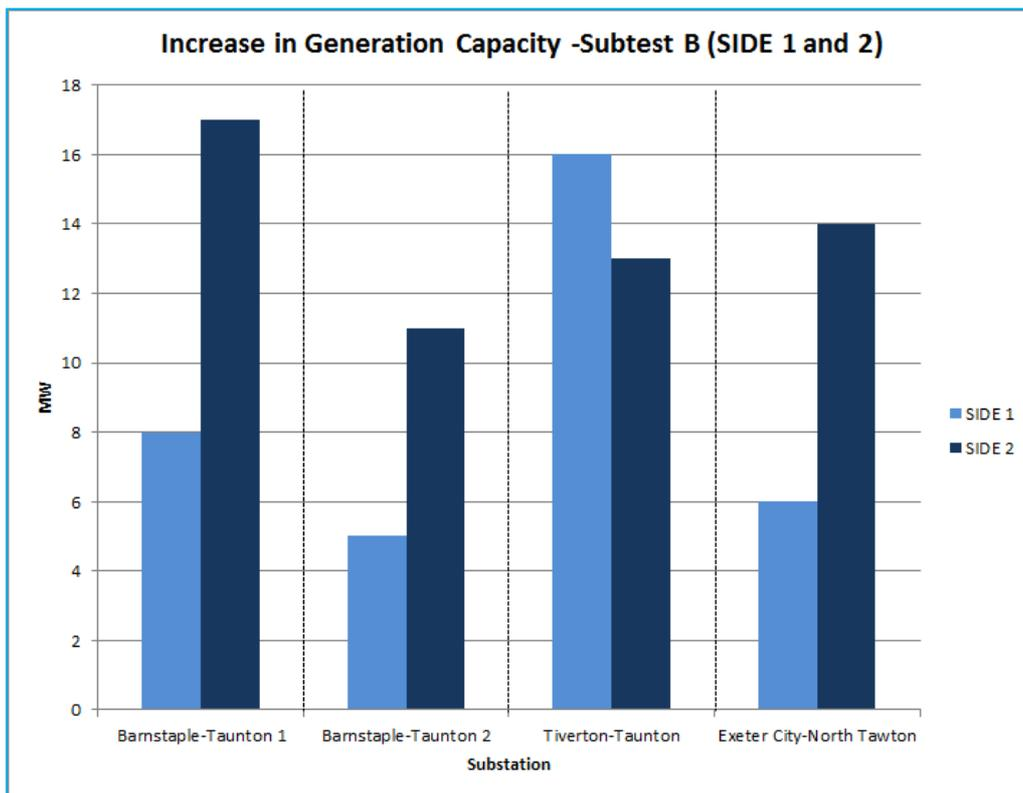
Figure 6-5: Increase in generation capacity flexibility using FPL
