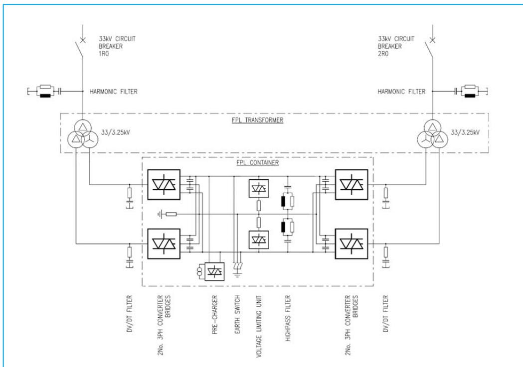
**Figure 2-5: FPL Electrical Single Line Diagram**
