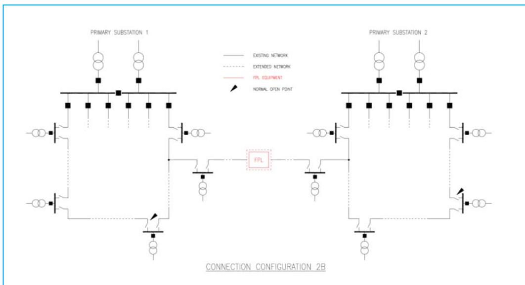
**Figure 8-3: Connection Configuration 2B SLD**
