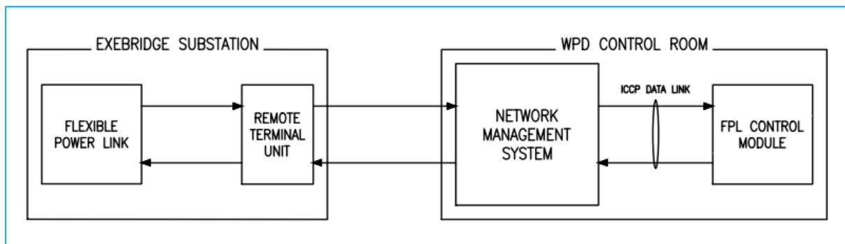
Figure 2-1: Overview of FPL System Architecture
