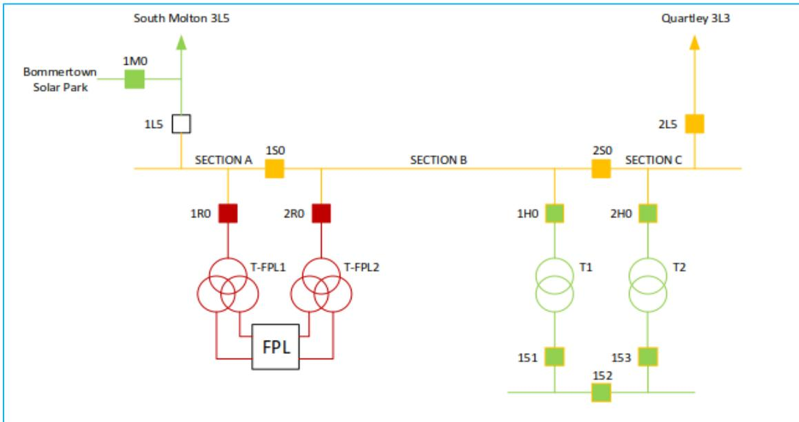
Figure 5-10: Bypass network configuration used for hot commissioning tests
