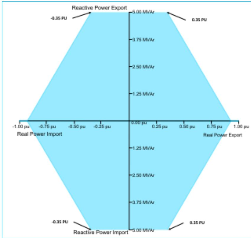
Figure 2-2: FPL Functional Specification Operating Window
