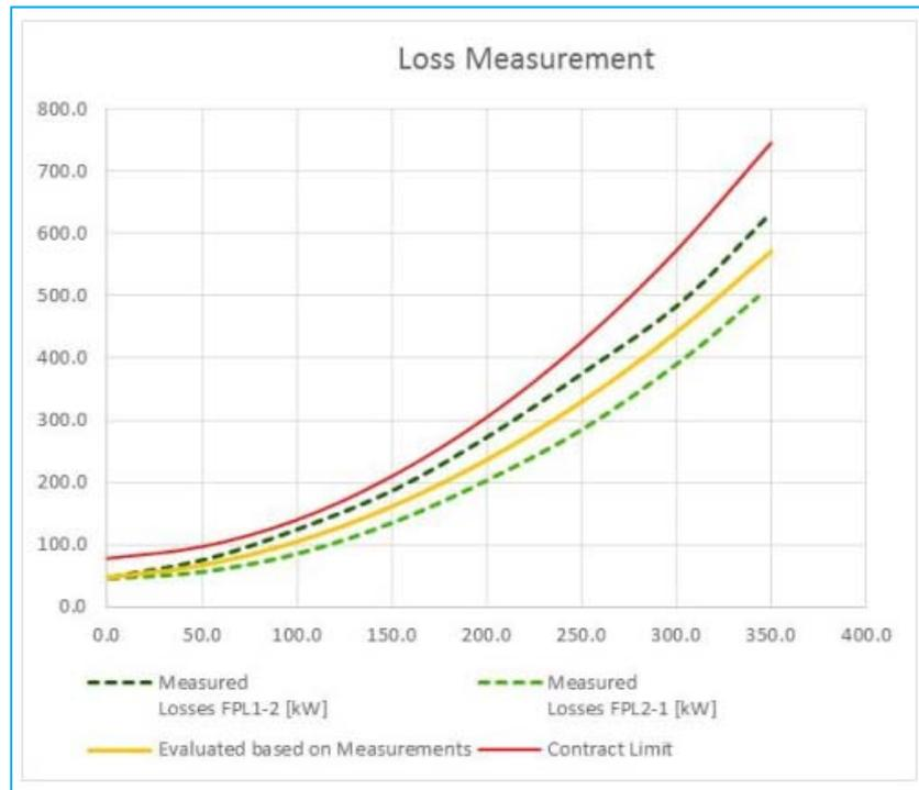
**Figure 5-13: FPL Loss Measurement Test Result**
