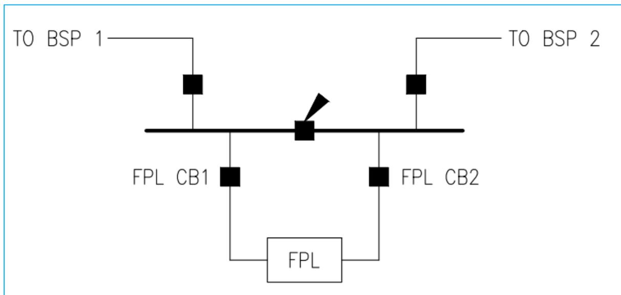
Figure 7-1: Proposed FPL Connection Method
