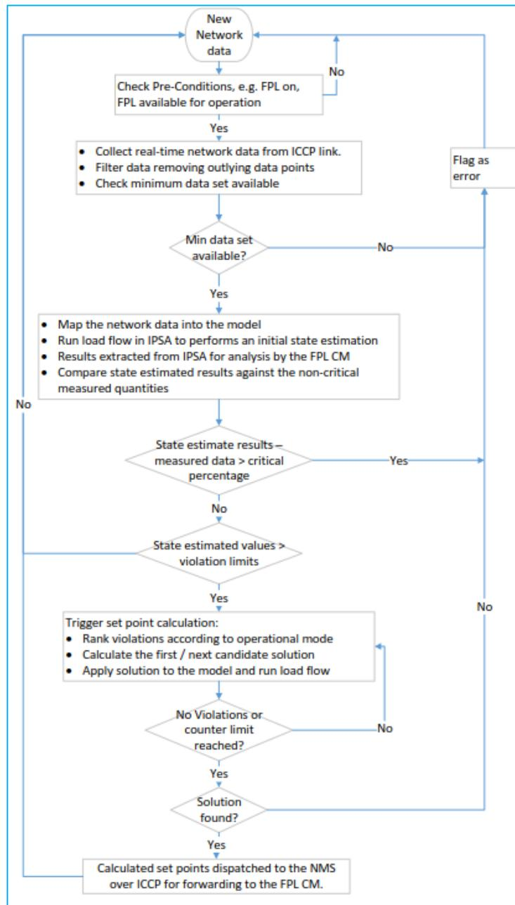
Figure 2-24: Overview of FPL CM Logic Sequence
