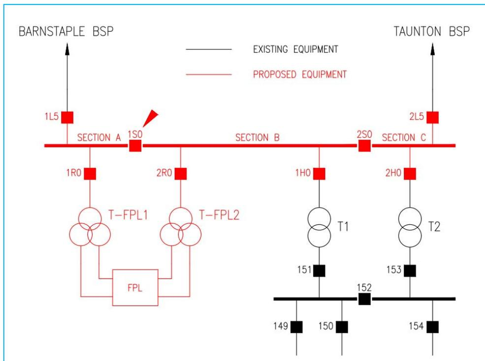
Figure 3-9: Exebridge Single Line Diagram for FPL Installation
