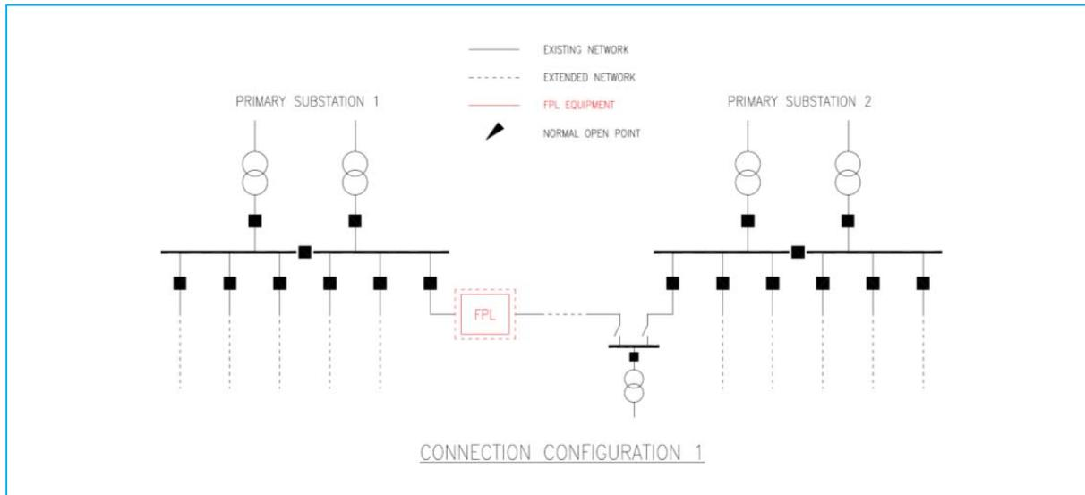
Figure 8-1: Connection Configuration 1 SLD
