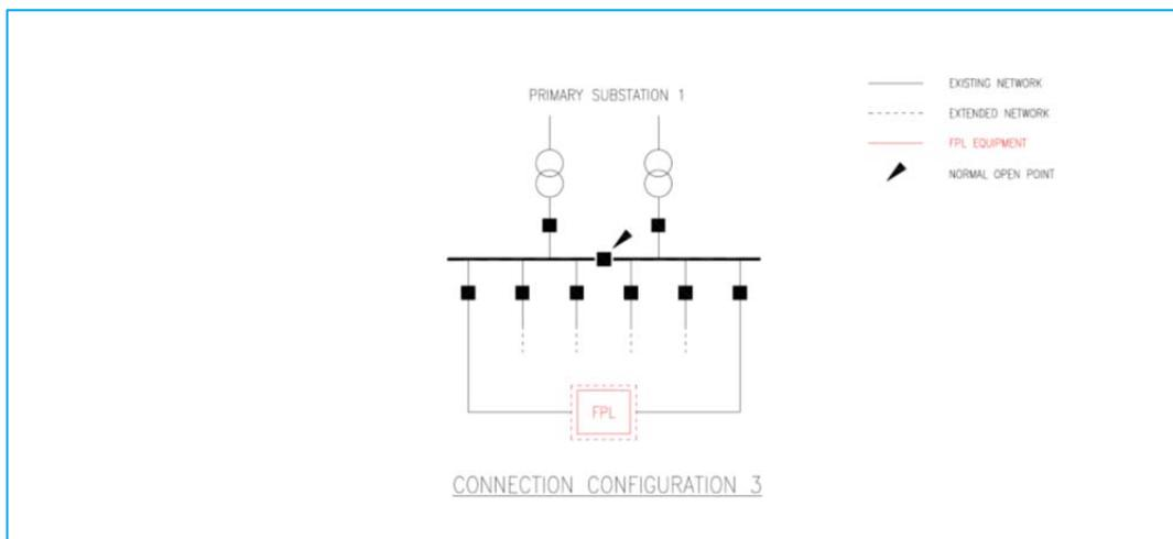
Figure 8-4: Connection Configuration 3 SLD
