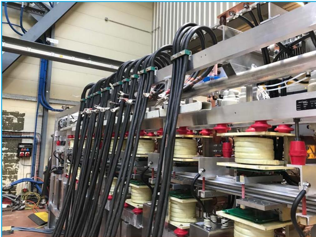
Figure 4-1: FCL Converter under Test
