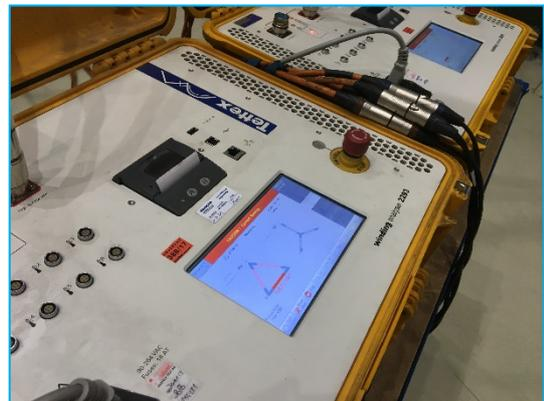
Figure 4-12: Winding resistance test
