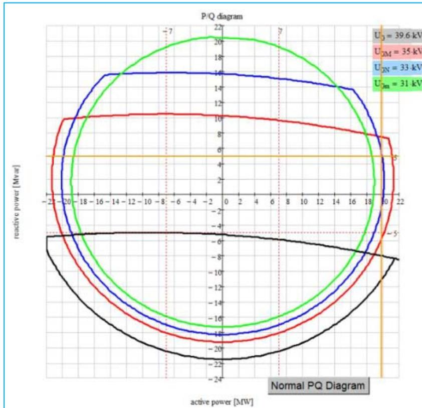
**Figure 5-14: FPL Power Capability Graph from Site Acceptance Testing**
