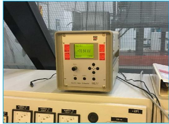
Figure 4-10: 70kV applied voltage test
