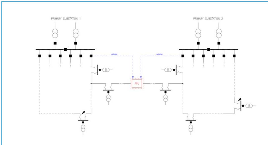
Figure 8-9: Example of intertripping for 11kV FPL
