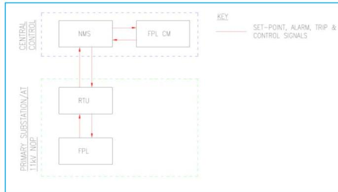
**Figure 8-6: FPL Control Module interface - Configurations 1 and 2**
