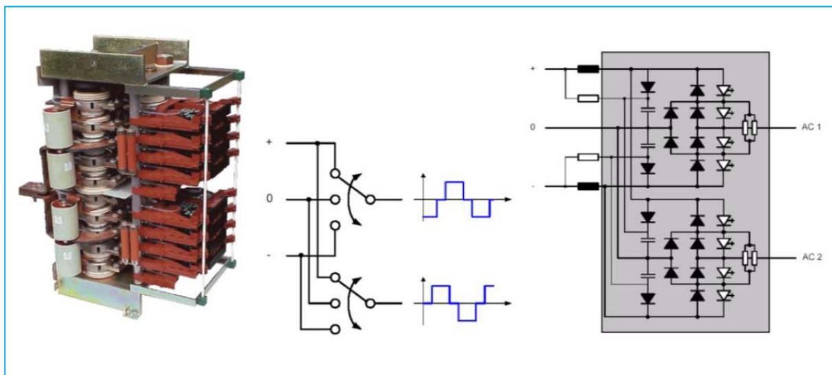
Figure 2-7: Power Electronic AC-DC Conversion
