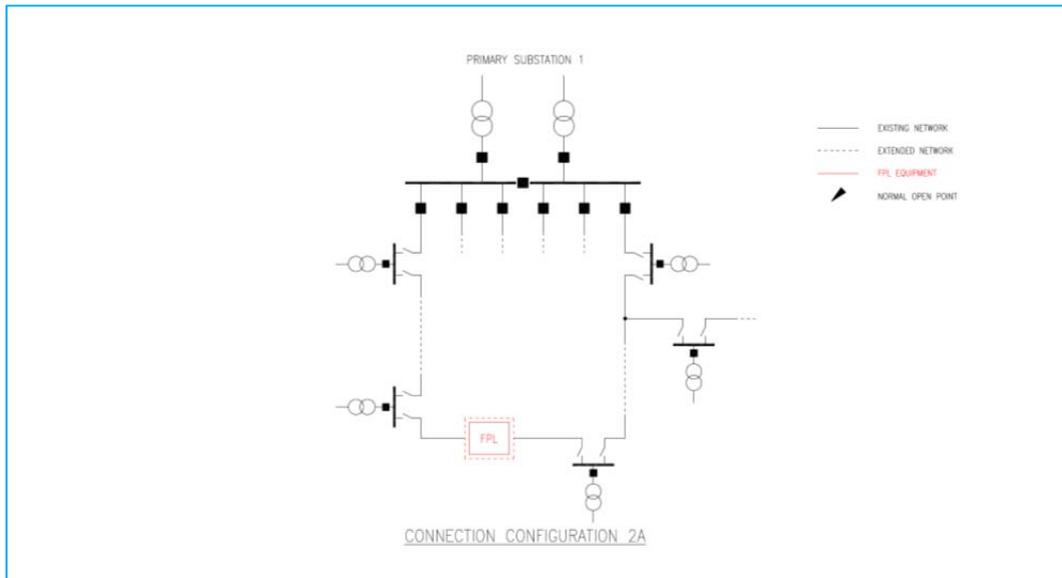
**Figure 8-2: Connection Configuration 2A SLD**
