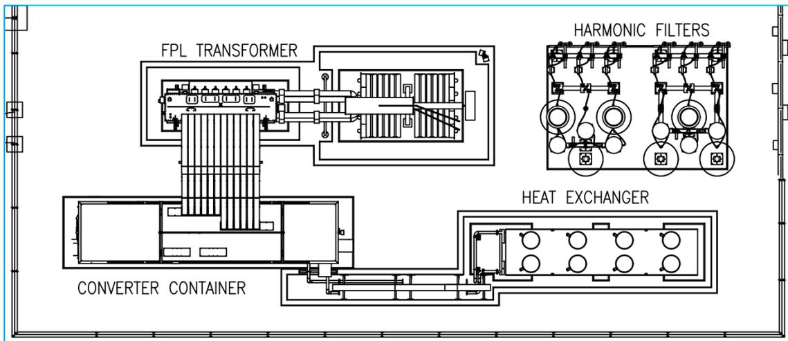
Figure 3-3: Final FPL Layout at Exebridge Substation
