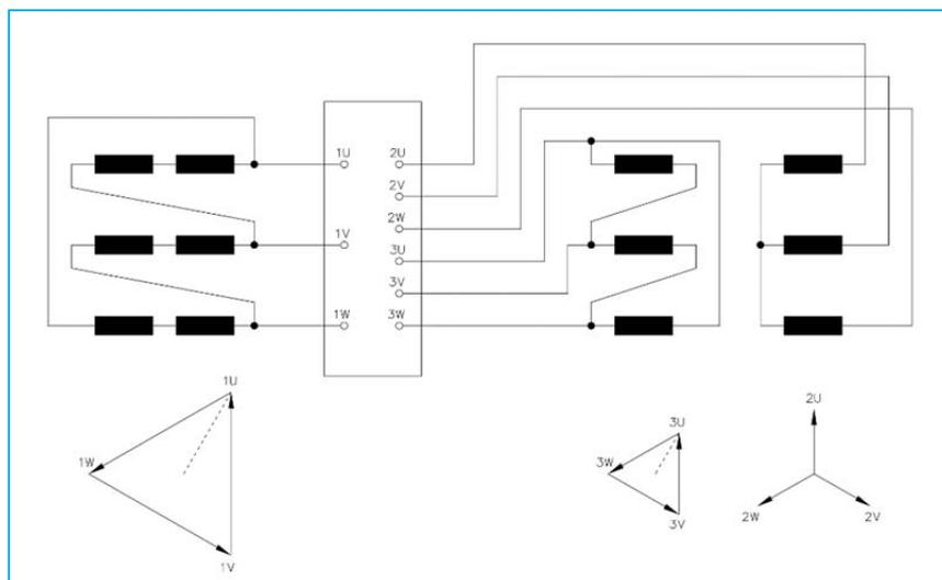
**Figure 2-11: FPL winding configuration for Transformer 1**
