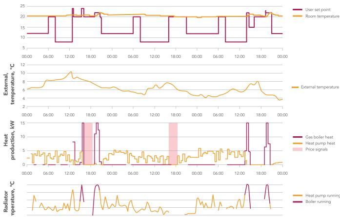
Figure 16: Case study showing time-series of a hybrid heating system with LPG, configured with a very high gas cost ratio matching real pricing in cold weather
