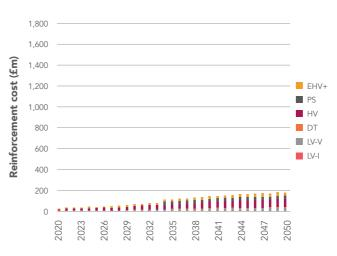
Figure 32: Development of South Wales' electricity distribution network upgrade cost for PassivSystems smart control of hybrids scenario
