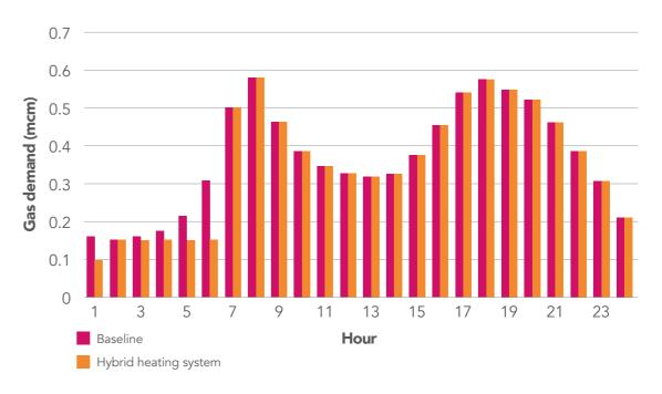
Figure 34: Hourly gas demand profiles for 'Baseline' and 'hybrid heating systems' scenarios
