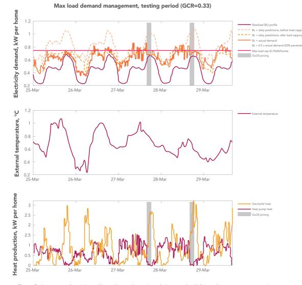
Figure 8: Aggregate electricity and heat demand over time during max load demand management operation, in a high gas price (GCR=0.33) scenario, involving 54 homes on average
