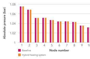
Figure 40: Pressure profile for LP#1 at 08:00 (peak) for different scenarios
