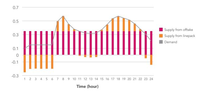
Figure 36: Gas supply and demand for the hybrid heating systems case
