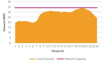
Figure 66: Local electricity demand at primary substation level and secured network capacity in a typical winter day
