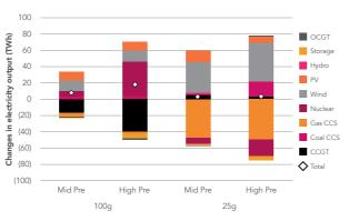
Figure 50: Implications of preheating on the energy mixes
