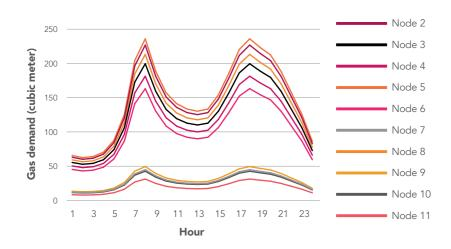
Given gas demand for the baseline and hybrid heating systems demand scenarios, gas flows along the pipes as well as nodal pressures were calculated for the whole time horizon (24 hours) to check whether the gas demand will be met without violating pressure limits.
