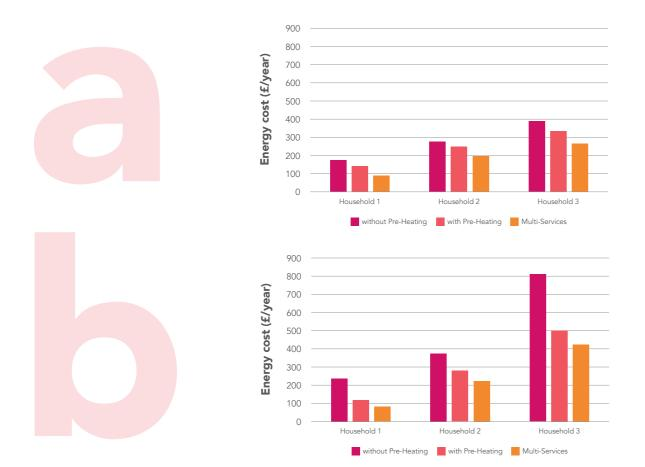
Figure 56: Energy costs when considering the provision of Multi-services (i.e. Pre-heating + Capacity + Balancing), considering different carbon targets for the energy sector (a) 100g CO./kWh, and (b) 25g CO./kWh. Households 1-3 increase from low to high heat demand
