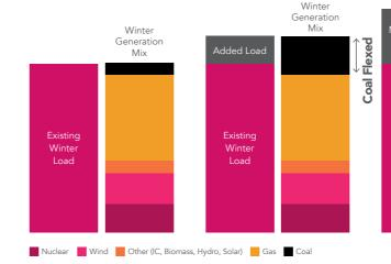
Figure 62: Illustration of generation sources meeting current power demand and added loads
