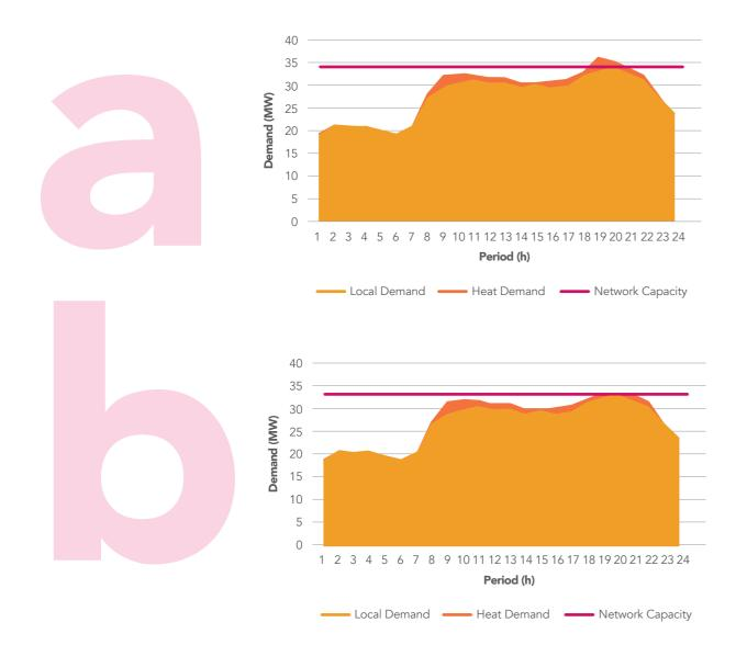
Figure 67: Local and electrified heat demand at the distribution network (a) without and (b) with network support service
