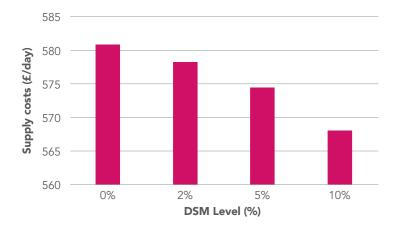
Figure 65: Heat supply cost associated with different levels of DSM
