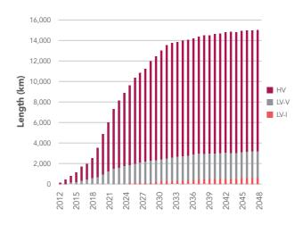
Figure 24: Development of South Wales's electricity distribution network upgrade (left) network length and (right) number of transformers for ASHP scenario; LV – low voltage network, DT – distribution transformer, HV – high voltage network, PT – primary transformer, I – thermal driven reinforcement, V - voltage driven reinforcement
