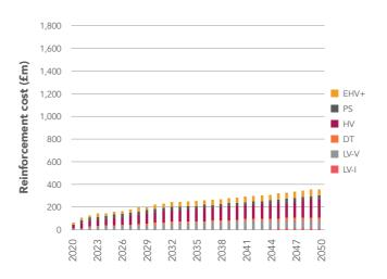
Figure 28: Development of South Wales's electricity distribution network upgrade cost for hybrid heating-only scenario
