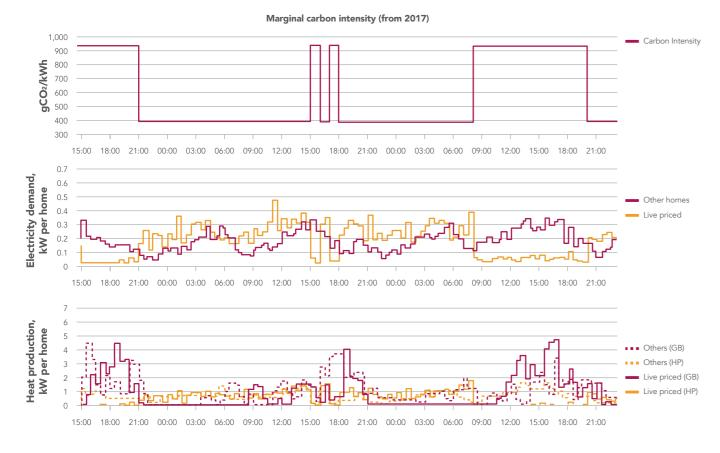
Figure 11: Aggregate electricity and heat demand over time in response to "marginal" carbon intensity price signals, on 22nd to 24th January 2018 (involving on average 13 live priced homes and 19 other homes).
