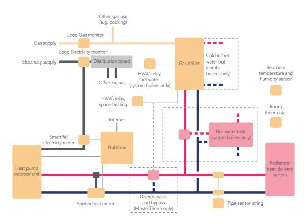
Figure 6: Schematic diagram of physical equipment deployed in a Freedom installation. Note that the Daikin configuration is different as the boiler and heat pump have a 'series' plumbing arrangement within the integrated unit
