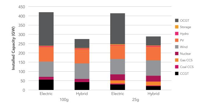
The results show that **the responsive hybrid heating system cases** require less firm generating capacity (needed for security reasons) than the capacity needed in the electric cases. It is noticeable that the capacities of open cycle gas turbines (OCGTs), combined cycle gas turbines (CCGT) and nuclear in the ASHP case are much higher than the corresponding capacities in the responsive hybrid heating system case.
