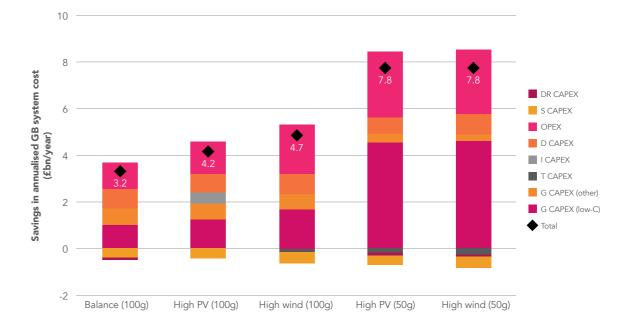
Figure 58: System-level benefits of flexible technologies
