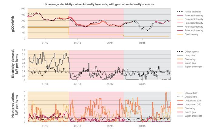
Figure 10 shows an aggregate electricity and heat demand over time in response to **electricity** day-ahead auction price signals on 16 and 17 January 2018 (involving on average 14 live priced homes and 19 other homes). The top line
