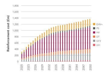
Figure 27: Development of South Wales's electricity distribution network upgrade cost for ASHP and hybrid heating scenario.
