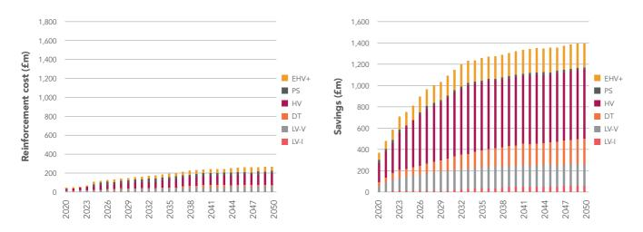
Figure 29: Development of South Wales' electricity distribution network upgrade cost for hybrid heating Economy Tariffs scenario.
