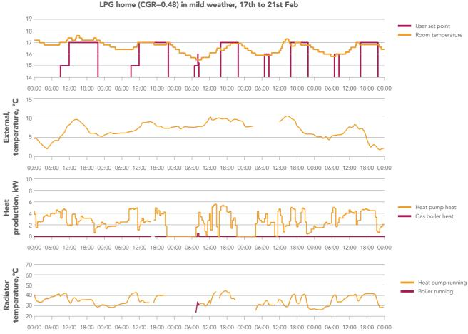
Figure 15: Case study showing time-series of a hybrid heating system with LPG, configured with a very high gas cost ratio matching real pricing, during typical winter weather
