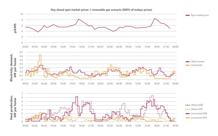
Figure 10: Aggregate electricity and heat demand over time in response to electricity day-ahead auction prices signals on 16 and 17 January 2018 (involving on average 14 live priced homes and 19 other homes)
