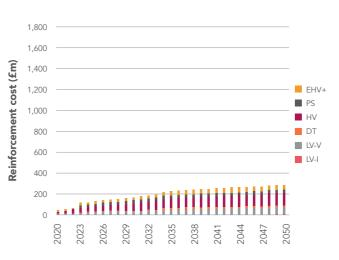
Figure 31: Development of South Wales' electricity distribution network upgrade cost for hybrid heating demand response scenario
