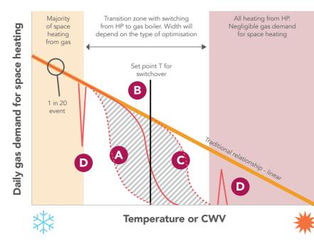
Figure 77: Hybrid heating system impact on gas demand
