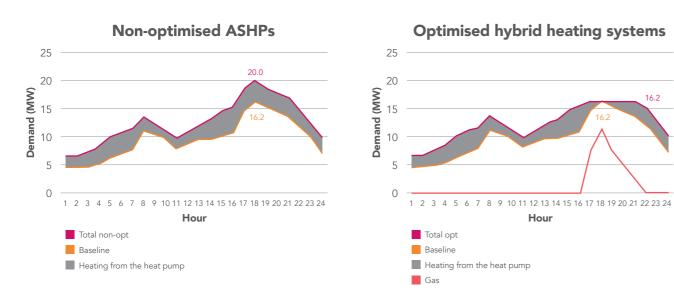
Figure 22: Non-optimised vs. PassivSystems' optimised hybrid heating system profiles
