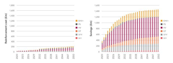
Figure 30: Development of South Wales' electricity distribution network upgrade cost for hybrid heating DUoS Tariff scenario
