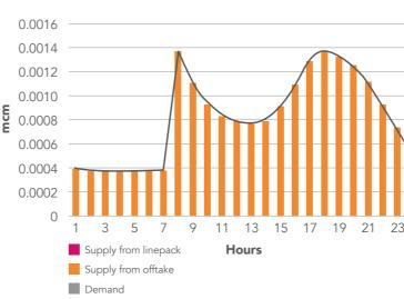
Figure 39: Gas supply and demand in the presence of hybrid heating systems
