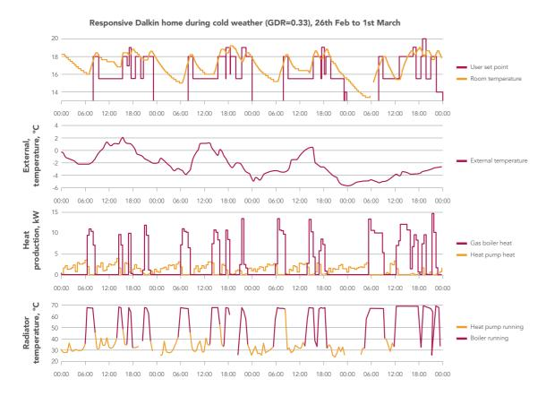
Figure 12: Case study showing time-series of a hybrid heating system during cold weather, on a high gas cost ratio
