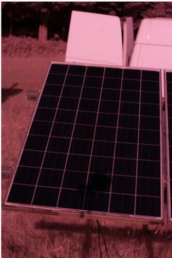
Figure 25: Infra-red image of a solar panel at night with no current flowing.
