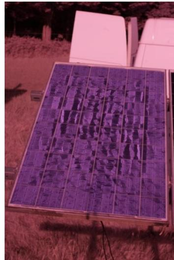
Figure 26: Infra-red image of a solar panel with reverse current applied at night.
