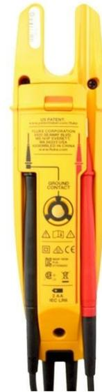
Figure 10: Rear view of Fluke T6 meter with non contact voltage detection
