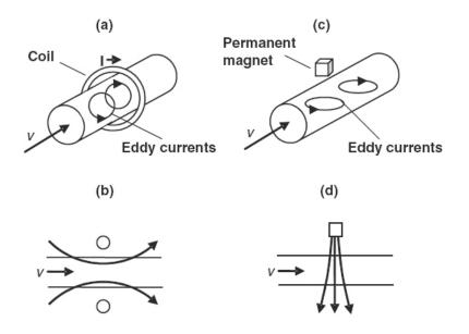
Figure 14: Lorentz flow meters – operating principle [15], and b are longitudinal and c and d are transvers methods
