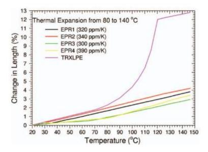
Figure 13: Change in length with temperature reproduced from Xiaoguang Qi and Steven Boggs "Thermal and Mechanical Properties of EPR and XLPE Cable Compounds" [14]
