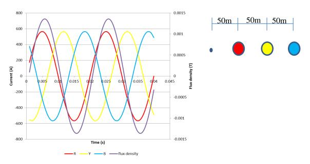
Figure 6 : Flux density in the presence of 3 balanced single core cables
