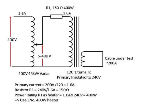
Figure 35: Simplified schematic of the test system used at Loughborough University. Note that earthing and protection is omitted in this drawing.
