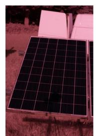
Figure 25: Infra-red image of a solar panel at night with no current flowing.
