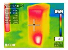
Figure 27: Thermal image of an LV feeder pillar.
