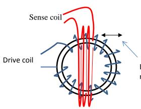
Fluxgate magnetometer – A drive coil is wrapped tightly round the coil. The sense coil does not go through the coil. The current required to drive the core into saturation one way versus the other way is compared to give a measure of flux density
