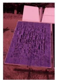
Figure 26: Infra-red image of a solar panel with reverse current applied at night.
