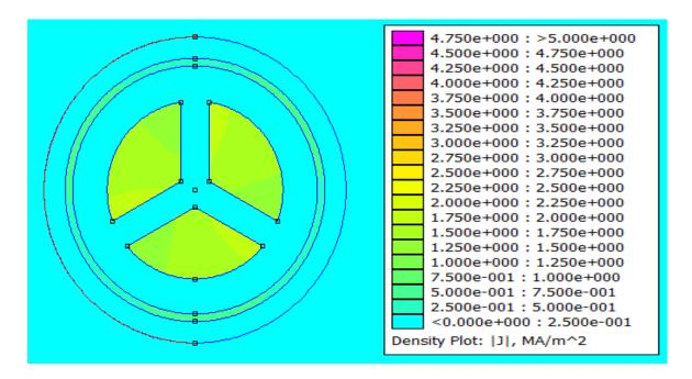
Figure 7 : Theoretical flux in a 3-core cable
