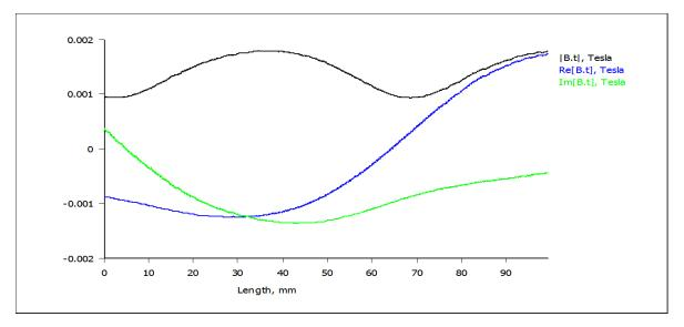
Figure 8 : Theoretical normal component of flux around the outside of a 3-core cable
