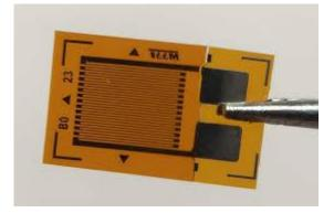
Figure 12: Example of a strain gauge
