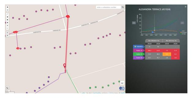
Figure 3: Example of mapped low voltage network showing over utilised cable segment highlighted
