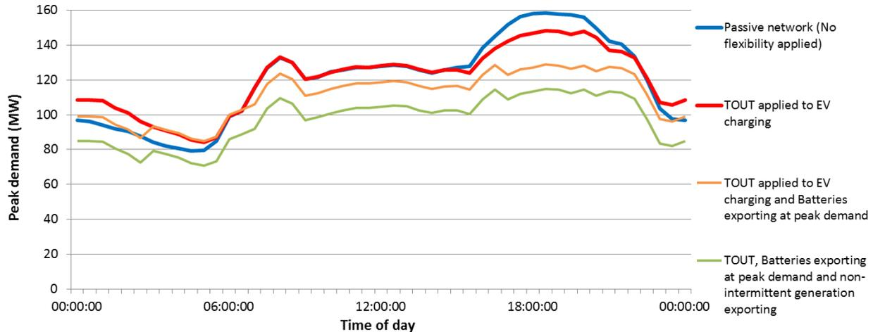
**Figure 19: Impact of flexibility and smart solutions on case study BSP for 2030 Two Degrees**
