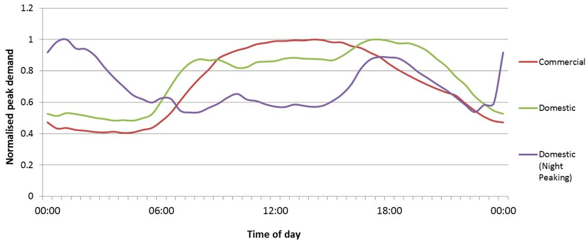
**Figure 3: Typical demand profiles for different BSP types**
