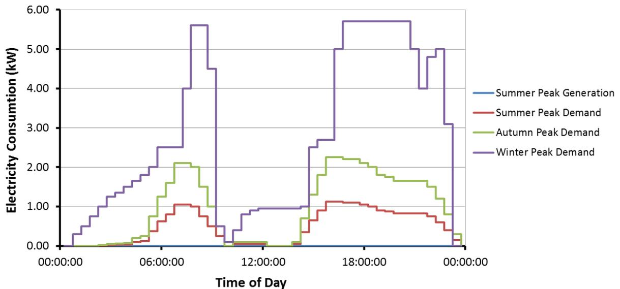
Figure 9: Electric back-up heat pump profile
