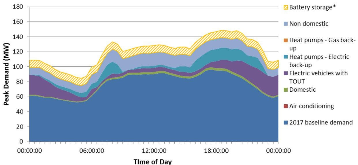
**Figure 15: WPD BSP day load profile for 2030 peak demand under the Two Degrees scenario with TOUT applied to EVs**
