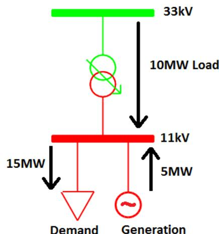
**Figure 1: Example showing the difference between demand and load**
