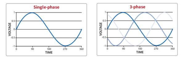
Three phase electricity is more commonly used in commercial and industrial connections. A good way of explaining the difference between single phase and three phase electricity is to imagine a paddler in a canoe. They can only move forward while their paddle moves through the water. When they lift the paddle out of the water to prepare for the next stroke, the power supplied to the canoe is zero.
