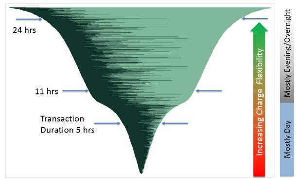
Figure 4.1: Electric Nation funnel diagram demonstrating spare charging capacity
