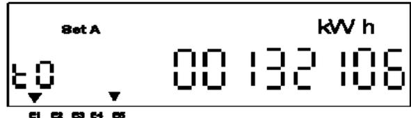
MD, Export, kVAh and kVArh registers are stored on Set B registers. They can be obtained by holding down the SELECT button for 3 seconds this switches the meter between Set A registers and Set B registers.
