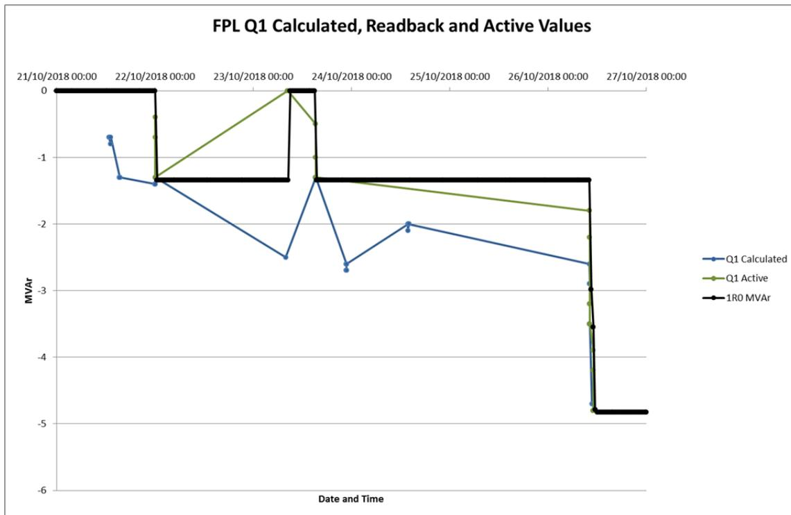
Figure 2-12: FPL operation to limit voltage rise (Q1)
