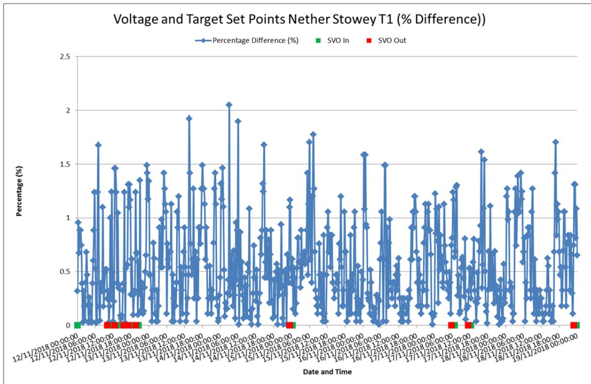
**Figure 2-3 Nether Stowey Primary (T1) voltage and set points % difference**
