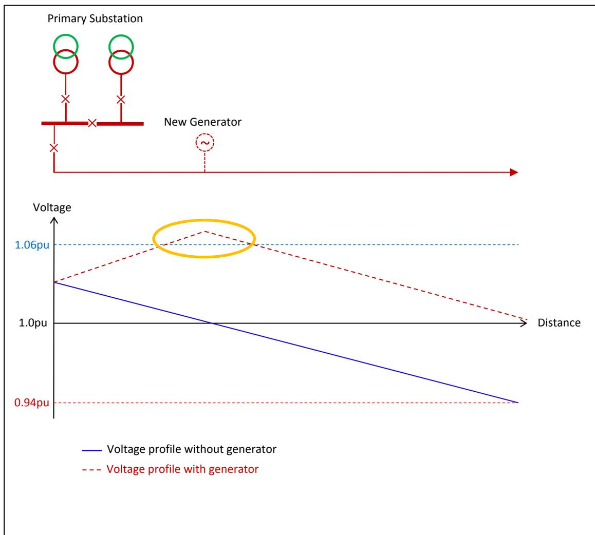
**Figure 1-1 - Impact on voltage from new generation connection**
