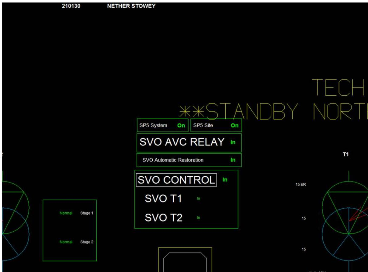
Figure 2-7 Automatic Restoration Indication in the NMS for Nether Stowey Primary
