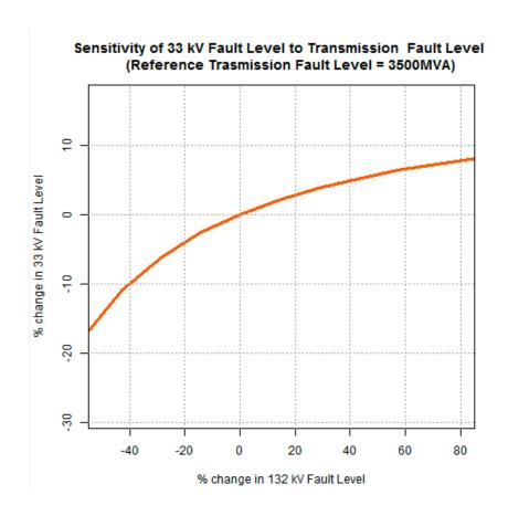
Decline in transmission upon distribution SCL is moderated by the impedance of the grid transformer
