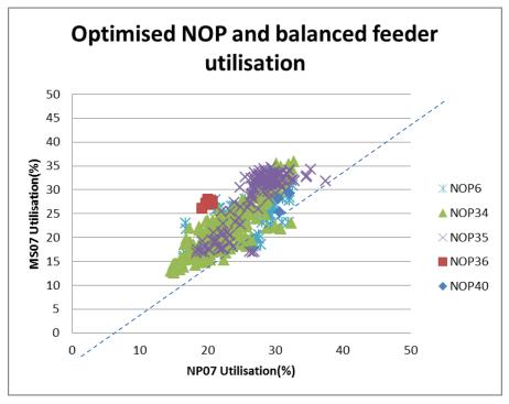
Figure 50 Feeder utilisation with optimised NOP between MS07 and NP07 (No. Hainault) Proportion of time at each NOP: NOP6-21.3%; NOP34-48.3%; NOP35-27.5% ; NOP36-2.3%; NOP40-0.6%
