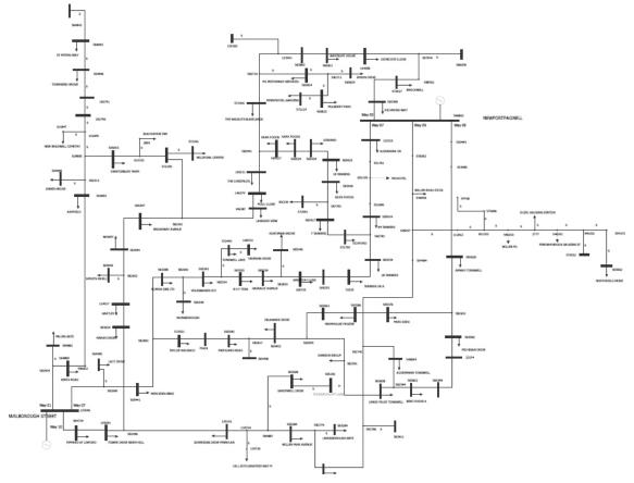
Figure 6: IPSA model for the Newport Pagnell and Marlborough Street substations
