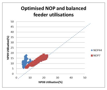
Figure 52: Feeder utilisation with optimised NOP between NP09 and NP08 (No. 7 Ackerman) Proportion of time at each NOP: NOP7-53.5%; NOP44-46.5%
