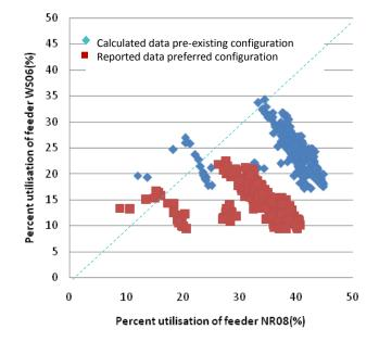
Figure 78: Feeder utilisation for week 2 (NR08/WS06)
