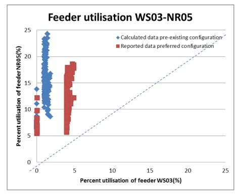
Figure 28: Measured and estimated feeder utilisation of WS03 and NR05 over week 2
