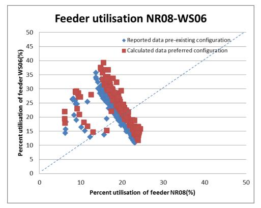
Figure 55: Measured and estimated feeder utilisation of WS06 and NR08 over week 1
