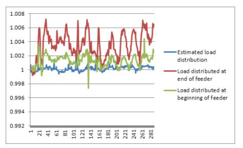
Figure 40 :Cable Network ratio (Ref#1/Ref#4)/( Ref#2/Ref#3) for each half hour slot over trial period
