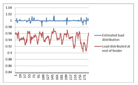
Figure 41 :OHL Network ratio (Ref#1/Ref#4)/( Ref#2/Ref#3) for each half hour slot over trial period
