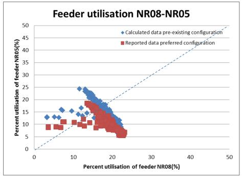
Figure 60 : Measured and estimated feeder utilisation of NR08 and NR05 over week 2
