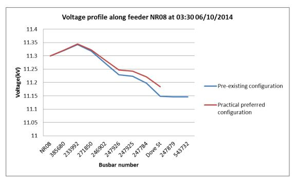
Figure 35 : Voltage profile along Newton Rd feeder 6 showing changes to voltage as the feeder is re-configured under method 1
