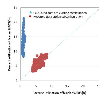
Figure 30: Feeder utilisation for week 2 (WS03/NR05)
