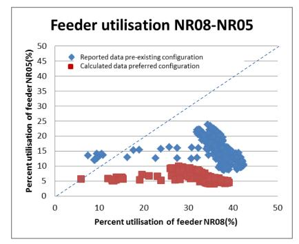
Figure 81 : Measured and estimated feeder utilisation of NR08 and NR05 over week 1
