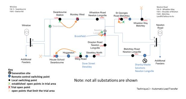
Figure 21: Stylised network diagram showing changes for network test starting 02/06/2015
