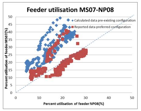
Figure 64: Measured and estimated feeder utilisation of MS07 and NP08 over week 2
