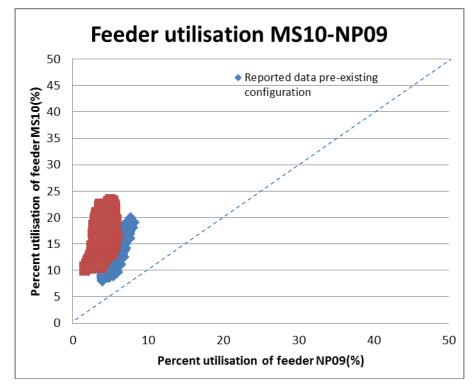
Figure 65: Measured and estimated feeder utilisation of MS10 and NP09 over week 1
