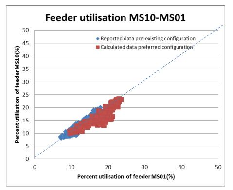
Figure 71 : Measured and estimated feeder utilisation of MS10 and MS01 over week 1
