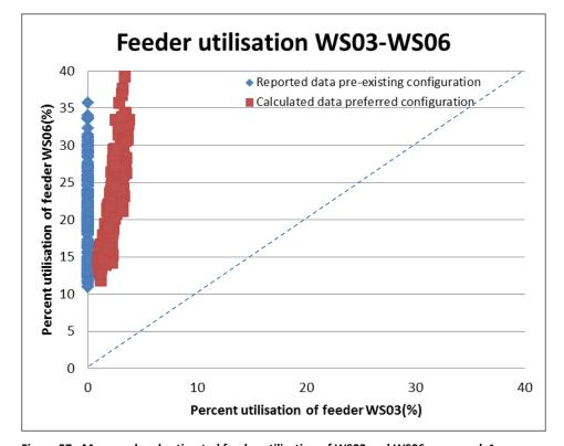
Figure 57 : Measured and estimated feeder utilisation of WS03 and WS06 over week 1
