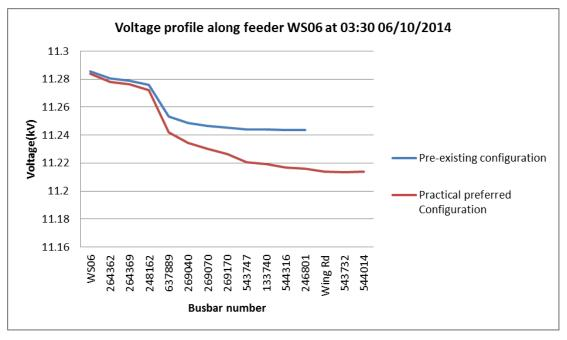
Figure 36 : Voltage profile along Winslow feeder 6 showing changes to voltage as the feeder is re-configured under method 1
