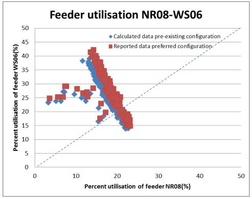
Figure 56: Measured and estimated feeder utilisation of WS06 and NR08 over week 2
