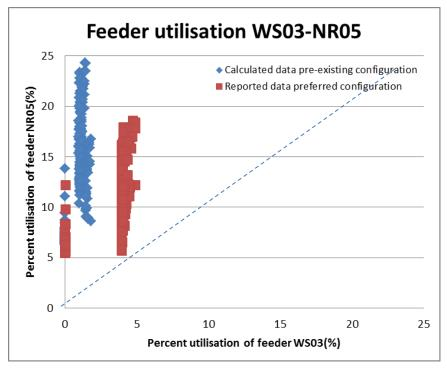
Figure 54: Measured and estimated feeder utilisation of WS03 and NR05 over week 2
