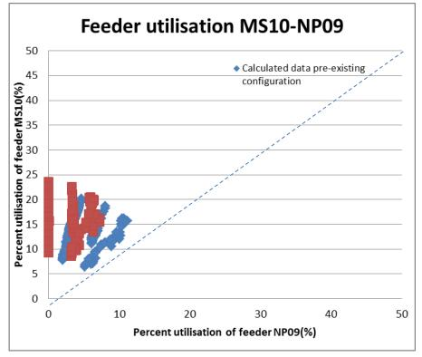
Figure 66: Measured and estimated feeder utilisation of MS10 and NP09 over week 2
