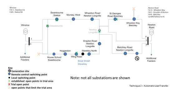
Figure 2: Stylised representation of the ALT overhead trial network
