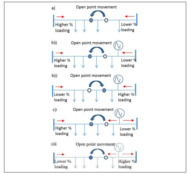
Figure 8 : NOP movement to balance feeder utilisation in the presence of a) load only, b) load and low value generation and c) load and high value generation.
