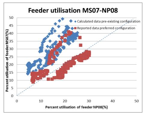
Figure 26: Measured and estimated feeder utilisation of MS07 and NP08 over week 2
