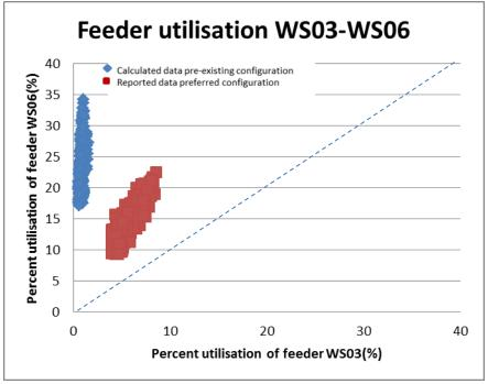
Figure 80 : Measured and estimated feeder utilisation of WS03 and WS06 over week 2
