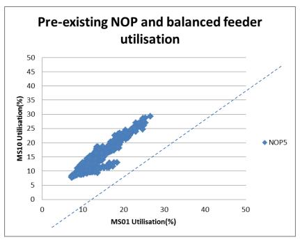
Figure 47: Feeder utilisation with pre-existing NOP between MS10 and MS01 (No.5 Wolverton Rd)
