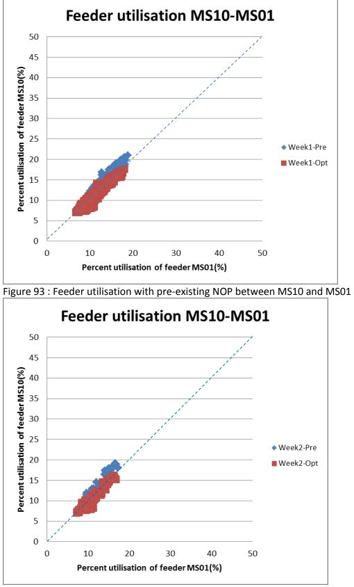
Figure 94 : Feeder customer utilisation with optimised NOP between MS10 and MS01
