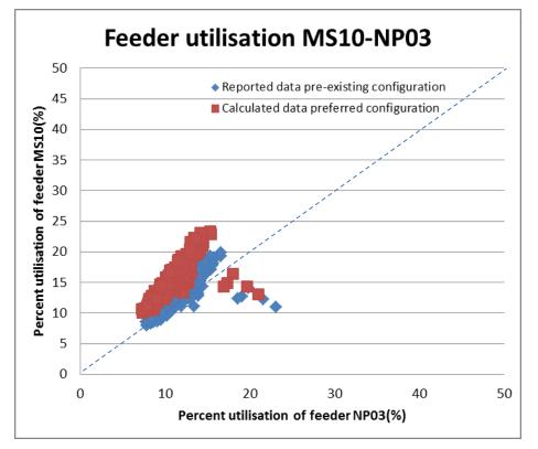
Figure 67 : Measured and estimated feeder utilisation of MS10 and NP03 over week 1
