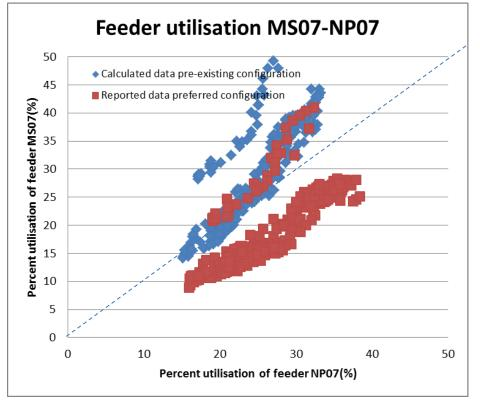
Figure 74 : Measured and estimated feeder utilisation of MS07 and NP07 over week 2
