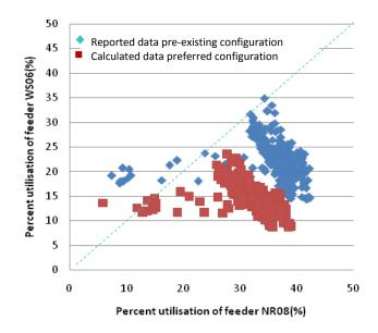
Figure 77: Feeder utilisation for week 1 (NR08/WS06)
