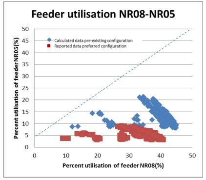
Figure 82 : Measured and estimated feeder utilisation of NR08 and NR05 over week 2
