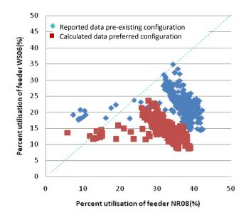
Figure 31: Feeder utilisation for week 1 (NR08/WS06)
