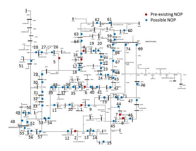
Figure 22: Illustration of possible NOP location for feeder utilisation balance on Cable trial network
