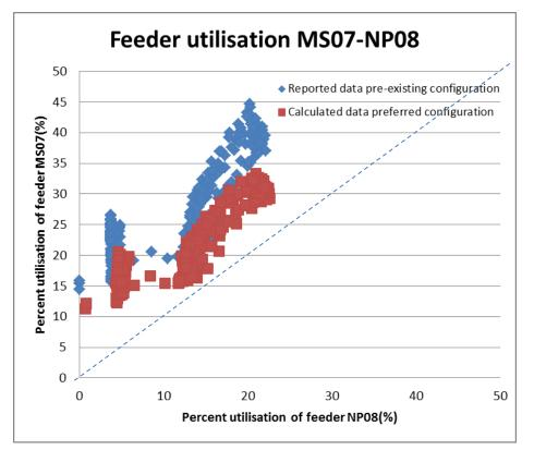
Figure 25: Measured and estimated feeder utilisation of MS07 and NP08 over week 1
