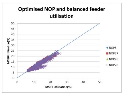
Figure 48: Feeder utilisation with optimised NOP between MS10 and MS01 (No.5 Wolverton Rd) Proportion of time at each NOP: NOP5-4.8%; NOP26-3.5%; NOP27-8.1%; NOP28-83.5%
