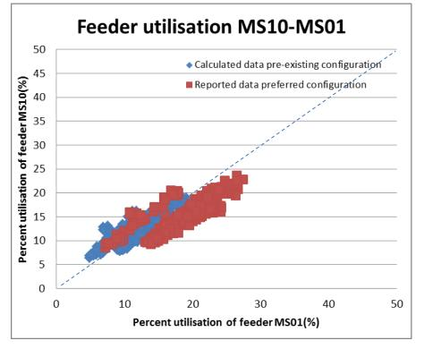
Figure 72 : Measured and estimated feeder utilisation of MS10 and MS01 over week 2
