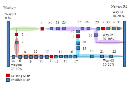
Figure 17 : Possible Open Point locations on OHL trial network using Method 2 analysis
