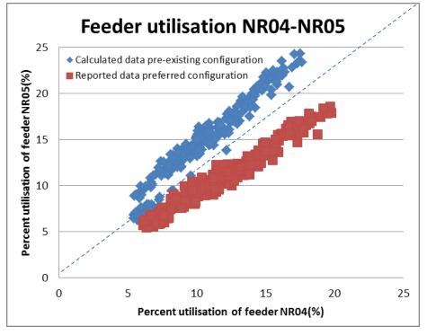
Figure 62 : Measured and estimated feeder utilisation of NR04 and NR05 over week 2
