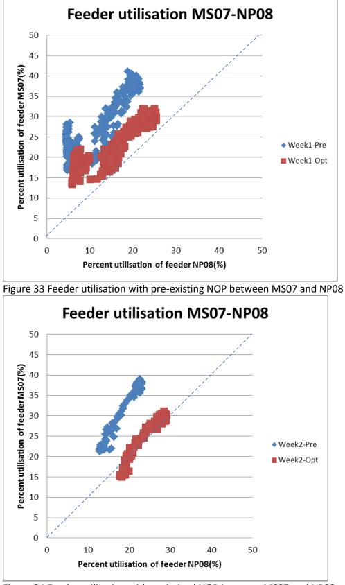
Figure 34 Feeder utilisation with optimised NOP between MS07 and NP08
