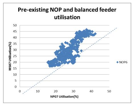
Figure 49: Feeder utilisation with pre-existing NOP between MS07 and NP07 (No.6 Hainault)
