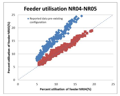
Figure 61 : Measured and estimated feeder utilisation of NR04 and NR05 over week 1
