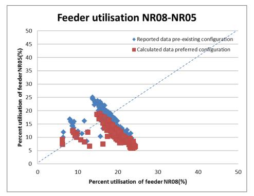
Figure 59 : Measured and estimated feeder utilisation of NR08 and NR05 over week 1
