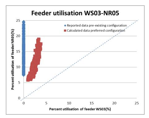
Figure 27: Measured and estimated feeder utilisation of WS03 and NR05 over week 1
