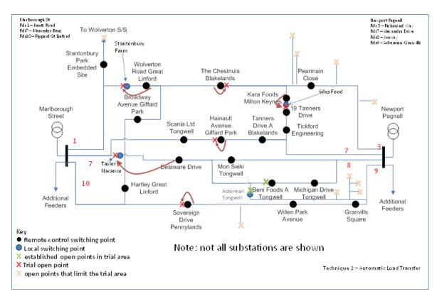
Figure 24: Stylised network diagram showing changes for network test starting 02/06/2015
