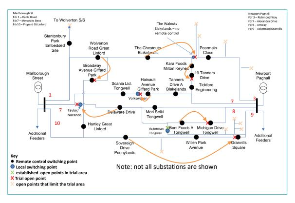
Figure 11: Stylised network diagram showing changes for 17-24 Jun - Configuration 1
