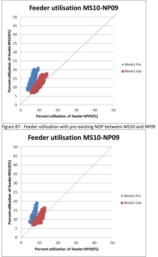
Figure 88 : Feeder utilisation with optimised NOP between MS10 and NP09
