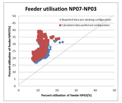
Figure 69 : Measured and estimated feeder utilisation of NP07 and NP03 over week 1
