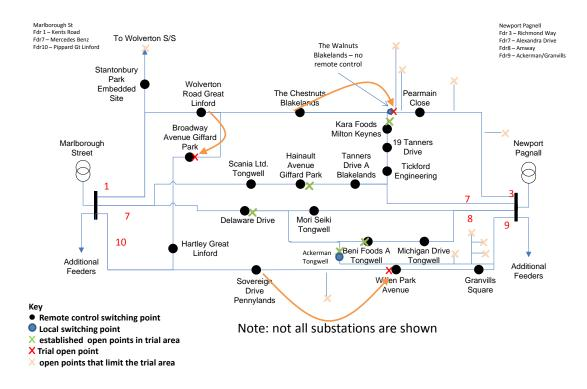
Figure 10 : Stylised network diagram showing changes for 22-29 May – initial test configuration
