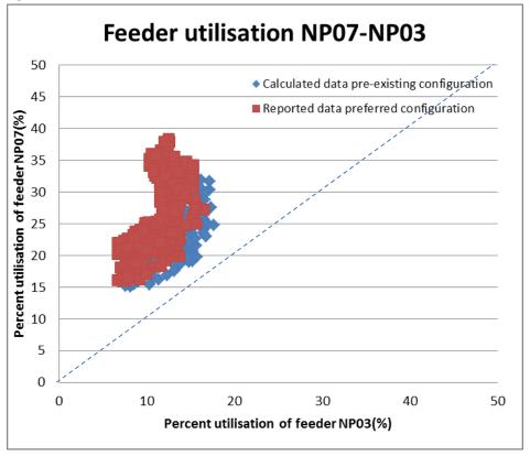
Figure 70 : Measured and estimated feeder utilisation of NP07 and NP03 over week 2
