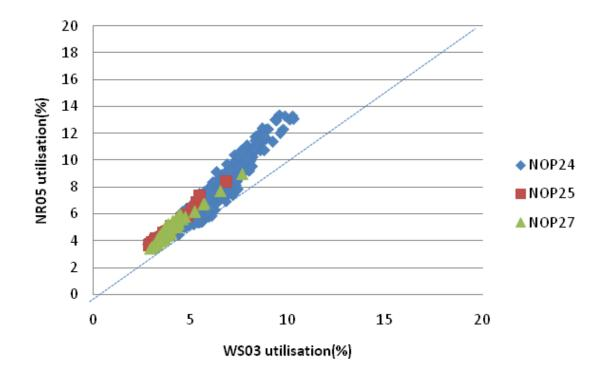
Figure 18 : Percentage Feeder utilisation of NR05 and WS03 over 10 typical days with calculated open point position
