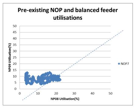
Figure 51: Feeder utilisation with pre-existing NOP between NP09 and NP08 (No. 7 Ackerman)
