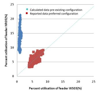
Figure 76: Feeder utilisation for week 2 (WS03/NR05)
