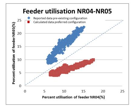
Feeder utilisation NR04-NR05 Calculated data pre-existing configuration Reported data preferred configuration Percent utilisation of feeder NR05(%) Percent utilisation of feeder NR04(%)
