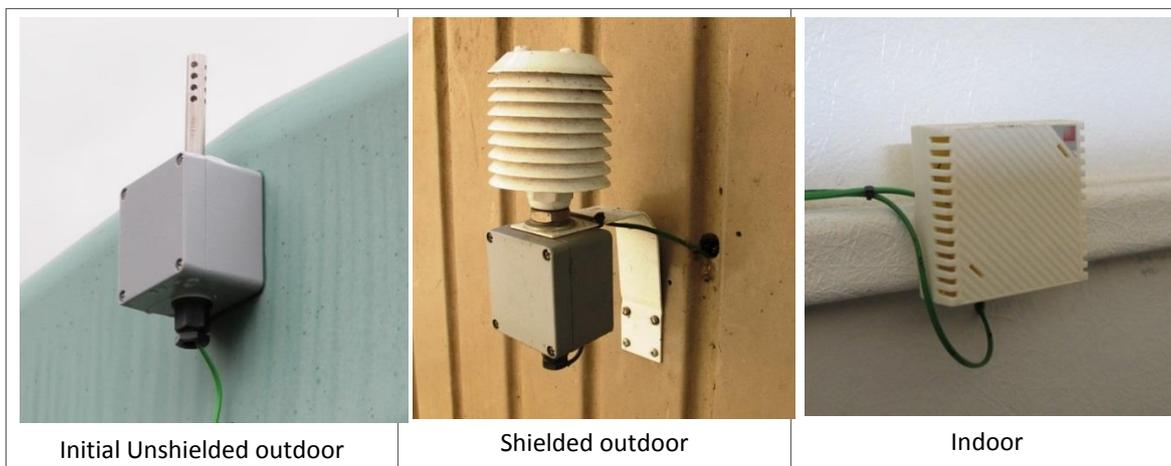
Figure 4 : Illustration of air temperature sensors, and positioning
