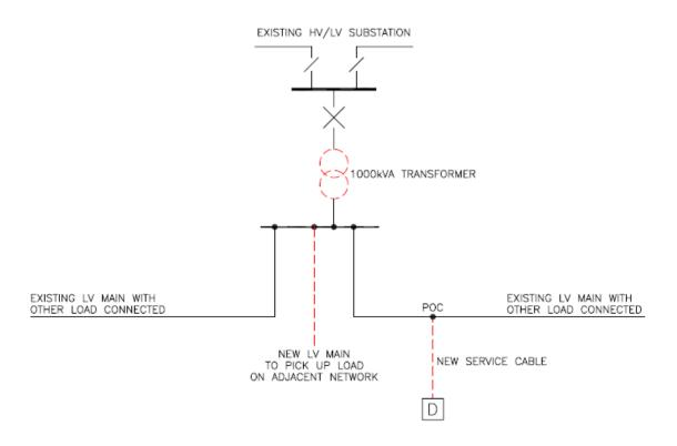
The RSN for the Reinforcement is the HV/LV transformer
