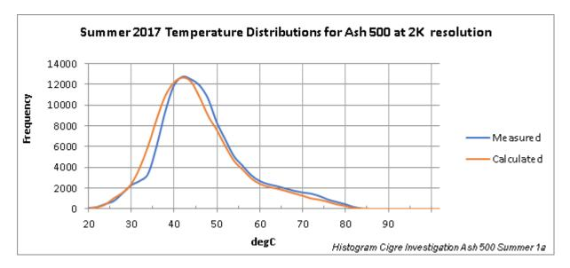
Figure 14 Frequency Distributions of Measured and Calculated Conductor Temperatures for the 2017 Summer (3 months) for Ash 500
