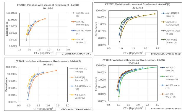
Figure 25 Same data as Figure 23 but with separate plot for each current. The four curves in each plot correspond to the four seasons. (Based on <u>provisional</u> design Tamb: 20-12-6-2)
