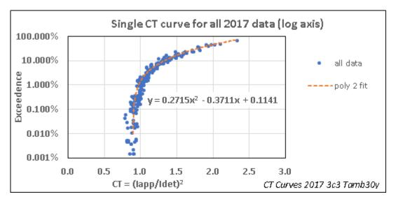
Figure 31 Similar curve to Figure 27 but with Tamb based on 30y UK averages and plotted as one single curve to enable curve fitting
