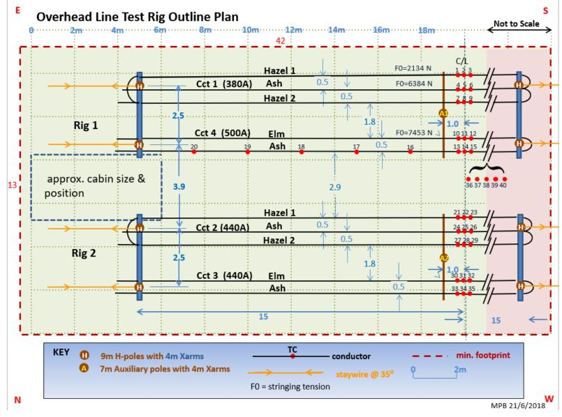
Figure 3 Overhead line test rig plan
