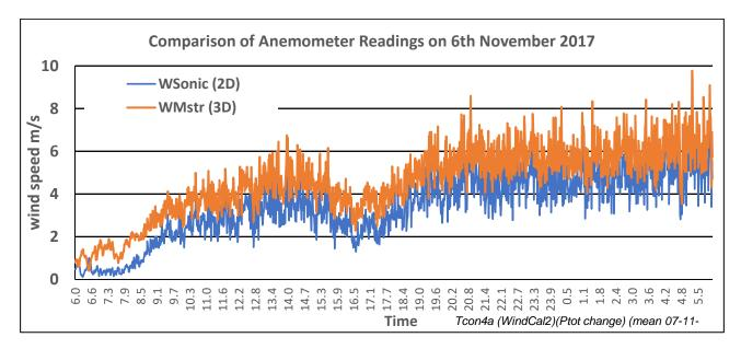
Figure 16 Discrepancy between the two anemometer readings
