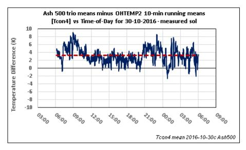
Figure 12 : 1-minute temperature difference (trio means minus calculated 10-minute running means) for the hottest conductor (Ash500) on a "high-temperature day" (29-30 October 2016)
