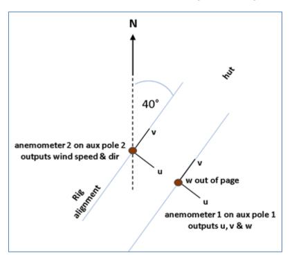
Figure 5 Diagram of overhead line & anemometer alignments
