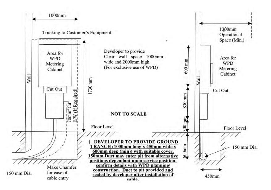
Note: Dimensions are suitable for most 4 and 7 solidal arrangements. The size may need to be increased where 11 solidals are installed depending on the number and direction of incoming ducts.
