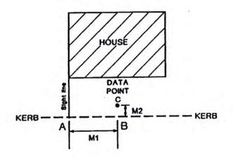
If there are no other deviations along its route, dimensions are taken at right angles to features if there position is known (interim points of deviation require additional dimensioning using method shown in example 4).
