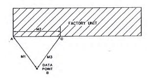
Here, two separate buildings can be used if it is the only alternative. Again, Points A and C are known requiring a measurement from each to confirm Point B (Data point).
