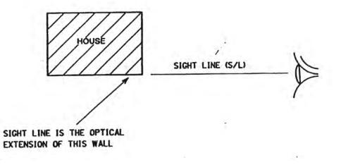
The position, once established, of the sight line on the ground, is confirmed by the placing of pegs, ranging rods, chain or tape measure.
