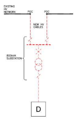
b) The Minimum Scheme is as for scenario a) above but the Customer requests an enhanced connection arrangement where the substation is looped into existing HV network.
