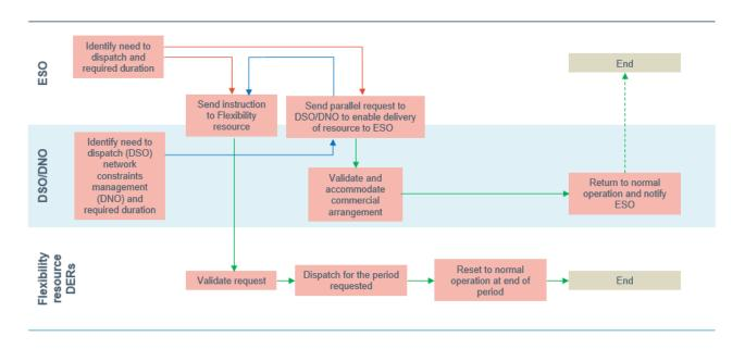
Figure 4-1: Overview of process associated with solution W1
