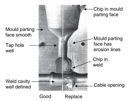
A CADWELD® mould is designed to last for an average of 50 connections. This will vary according to the care given to the mould during use.
