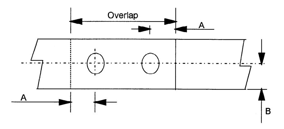
Figure 1 - Bolting Arrangement
