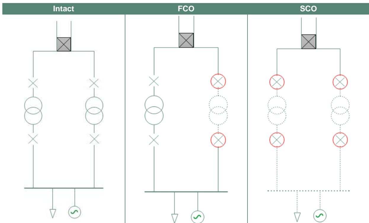
**Figure 1: Simplified power system diagram showing intact, FCO and SCO conditions at a substation**
