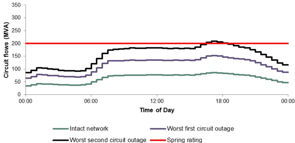
**Figure 5: Spring flows on circuit C calculated using time-step analysis**
