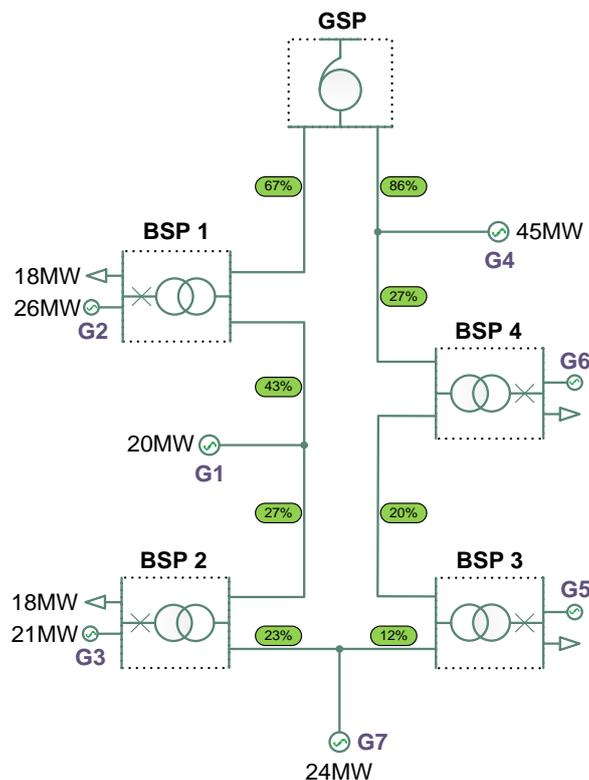
**Figure 7: Intact network showing circuit loadings with no generation constrained**
