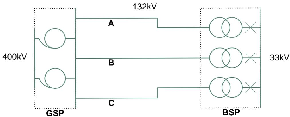
**Figure 3: Three circuit 132kV supply group**
