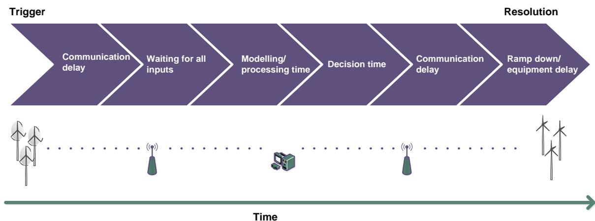
**Figure 6: Example of the delays seen when carrying out switching or generator curtailment with real-time analysis in the loop**
