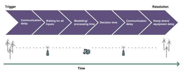
Figure 6: Example of the delays seen when carrying out switching or generator curtailment with real-time analysis in the loop
