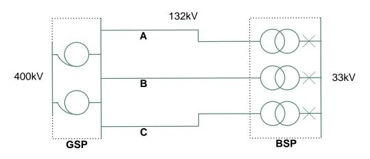
Figure 3: Three circuit 132kV supply group
