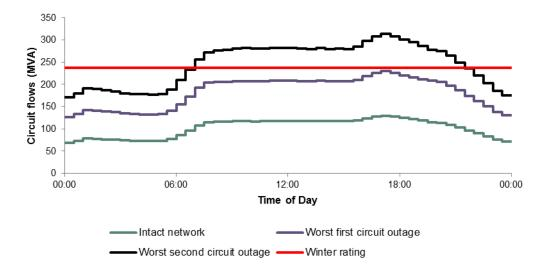
Figure 4: Winter flows on circuit C calculated using time-step analysis
