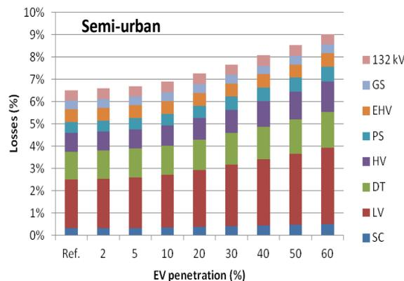
Figure 14: Impact of EV penetration on losses in semi-urban network; smart EV charging
