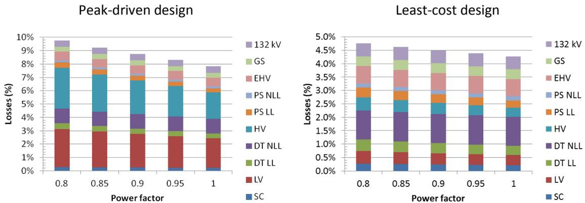
Figure 24: Variation of losses with PF in semi-rural network types
