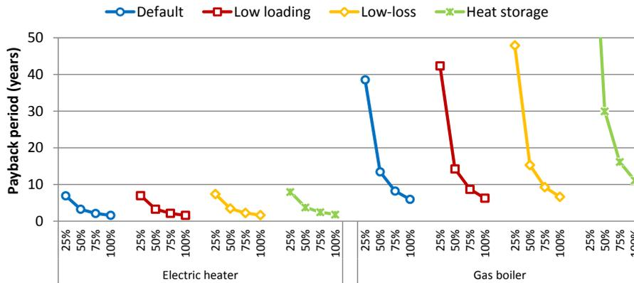
**Figure 41: Sensitivity of payback period to different assumptions on parameters of the heat recovery system**
