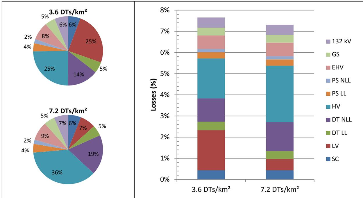
Figure 28: Impact of distribution transformers density on losses in a semi-rural type network
