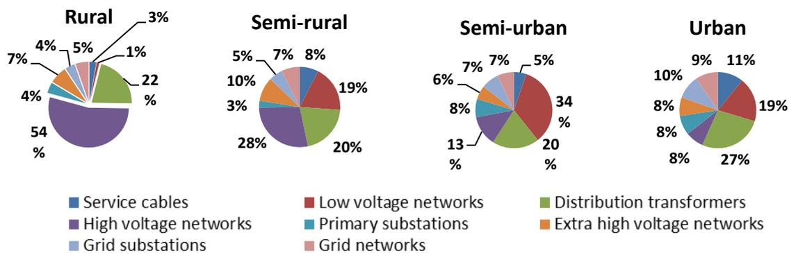
Figure 3: Breakdown of losses across distribution networks in four types of network
