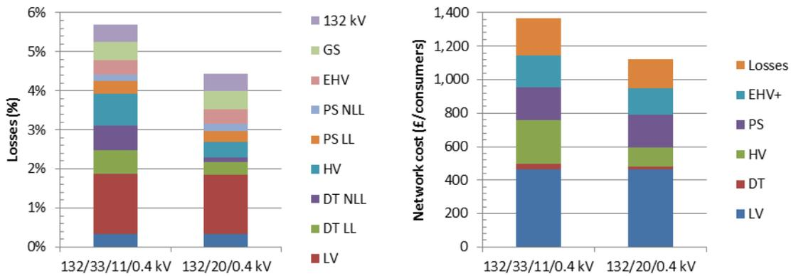
**Figure 33: Losses in distribution systems with various voltage levels; LV – low voltage, DT – distribution transformer, HV – high voltage, PS – primary substation, EHV – extra high voltage (33 kV), GS – grid substation, 132 kV – grid network, LL – load losses, NLL – no-load losses**
