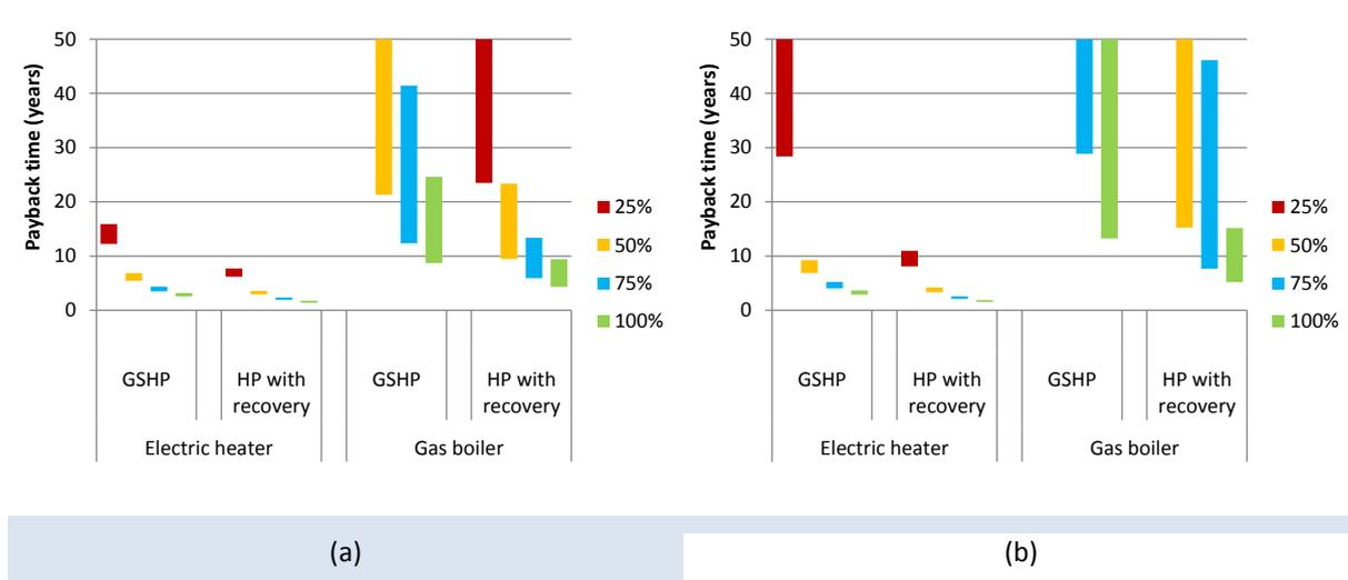
**Figure 39: Payback times for heat pump systems with and without heat recovery measured against electric heater and gas boiler, for discount rates of (a) 3% and (b) 9%**
