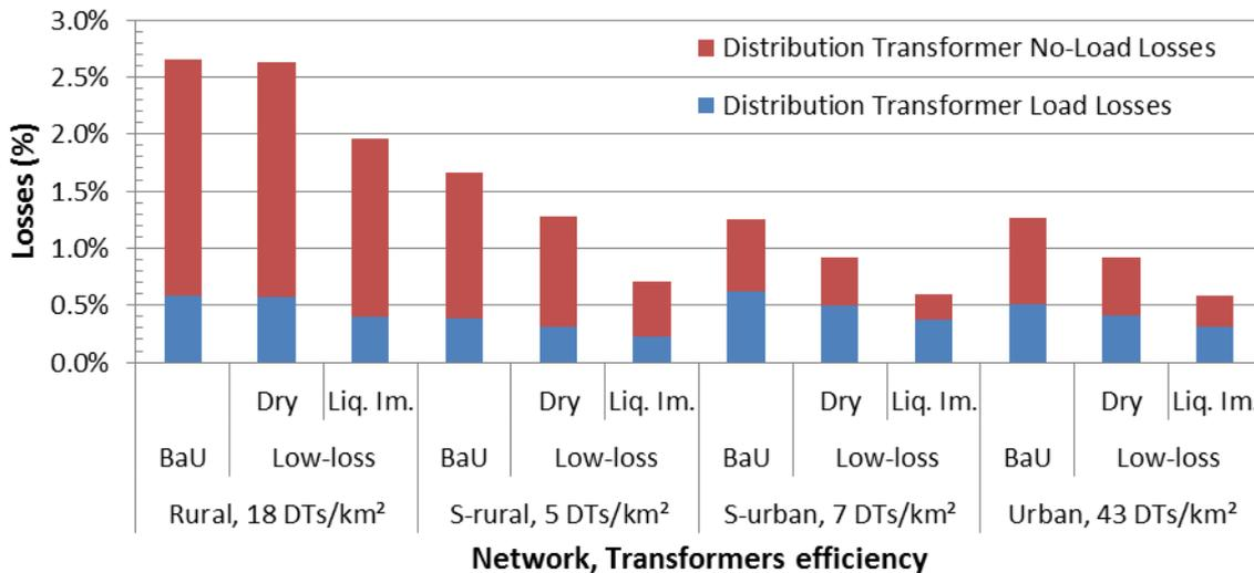
Figure 27: Comparison of overall transformer losses for standard and low-loss transformers
