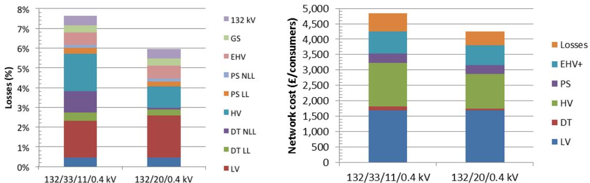
**Figure 34: Comparison of losses for four and three voltage level designs of semi-rural type networks**
