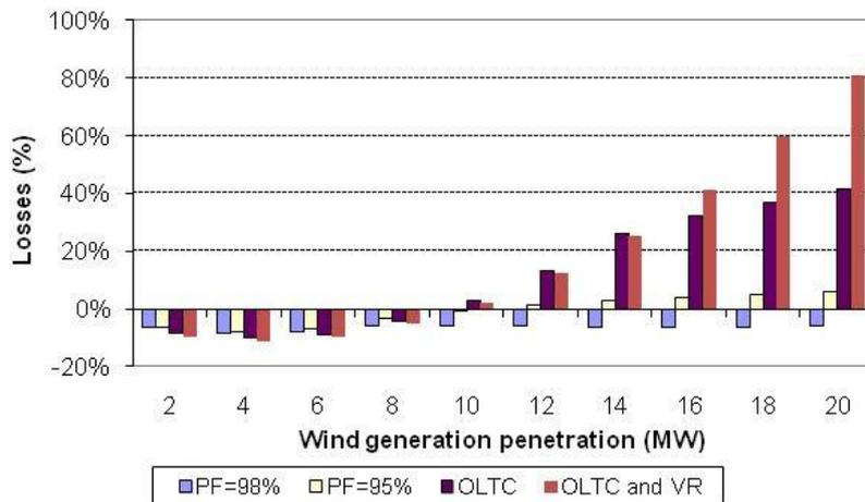
Figure 13: Impact of ANM schemes on network losses for various level of penetration of wind generation
