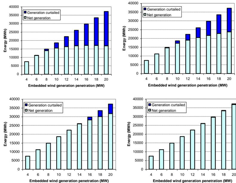
**Figure 12: Benefits of four alternative ANM schemes: 0.98 PF, 0.95 PF, Area based OLTC, Area based OLTC with in line voltage regulation**
