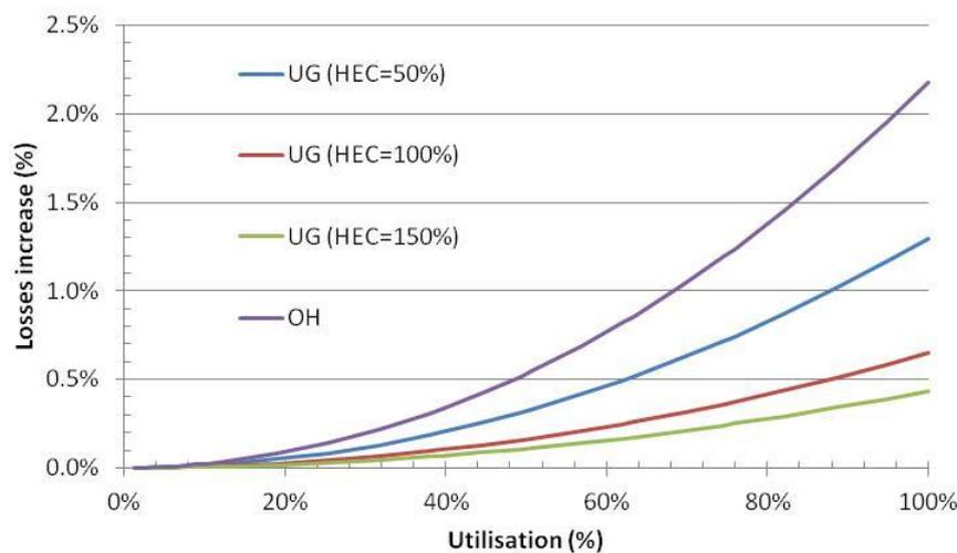
Figure 15: Impact of temperature on losses
