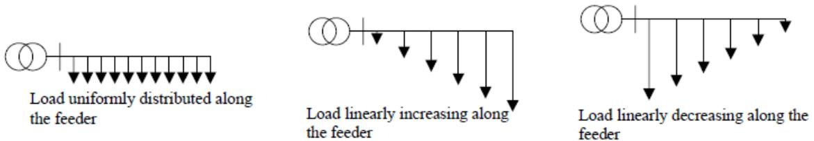
Figure 35: Load profiles assessed for the impact of cable tapering
