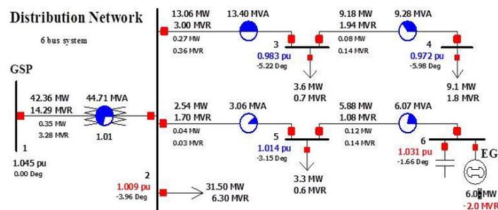
Figure 11: 33kV network model showing maximum loading conditions
