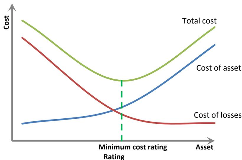
Figure 16: Impact of loss inclusive network design on asset costs
