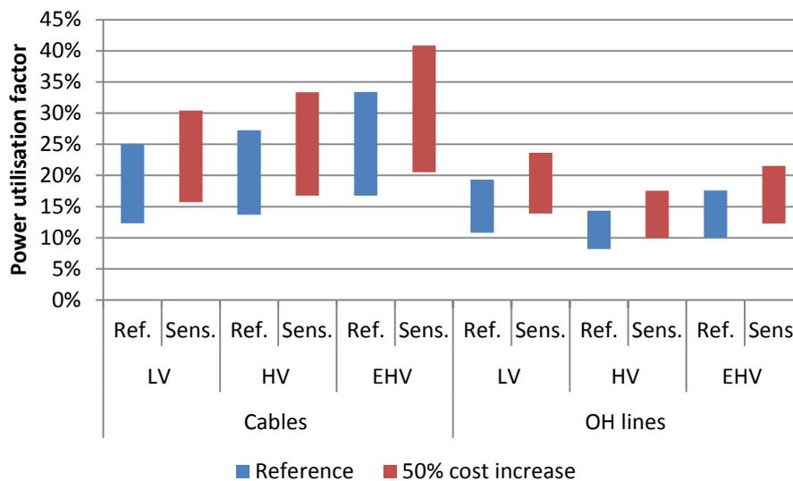
Figure 19: Sensitivity of power utilisation factor
