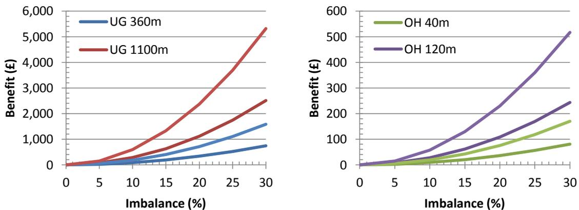
**Figure 5: Range of potential phase balancing benefits per feeders; minimum benefit is for discount rate of 9% over 20 years while maximum benefit is for discount rate of 3.5% over 45 years**
