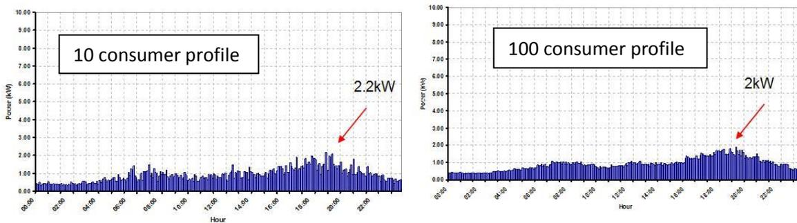
Figure 7: Diversified load profiles
