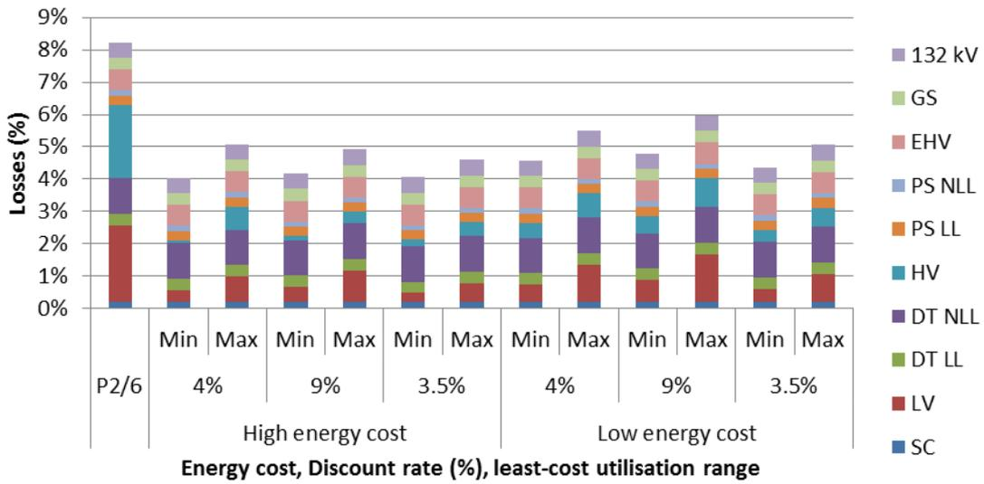
Figure 21: Least cost network design for semi-rural networks
