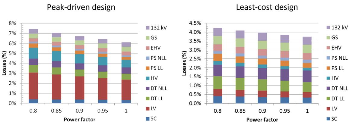
Figure 25: Variation of losses with PF in semi-urban network types
