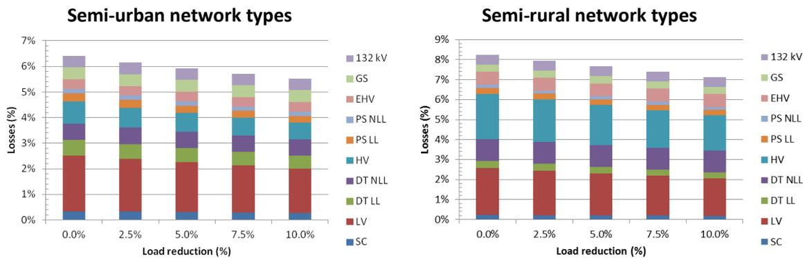
Figure 10: Impact of load reduction on network losses for semi-urban and semi-rural networks
