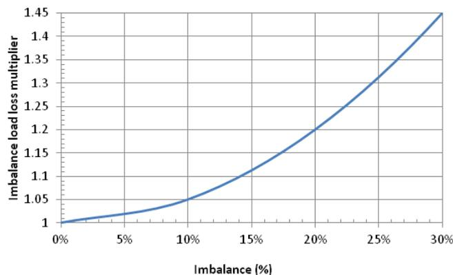
**Figure 4: Effect of phase imbalance on losses**
