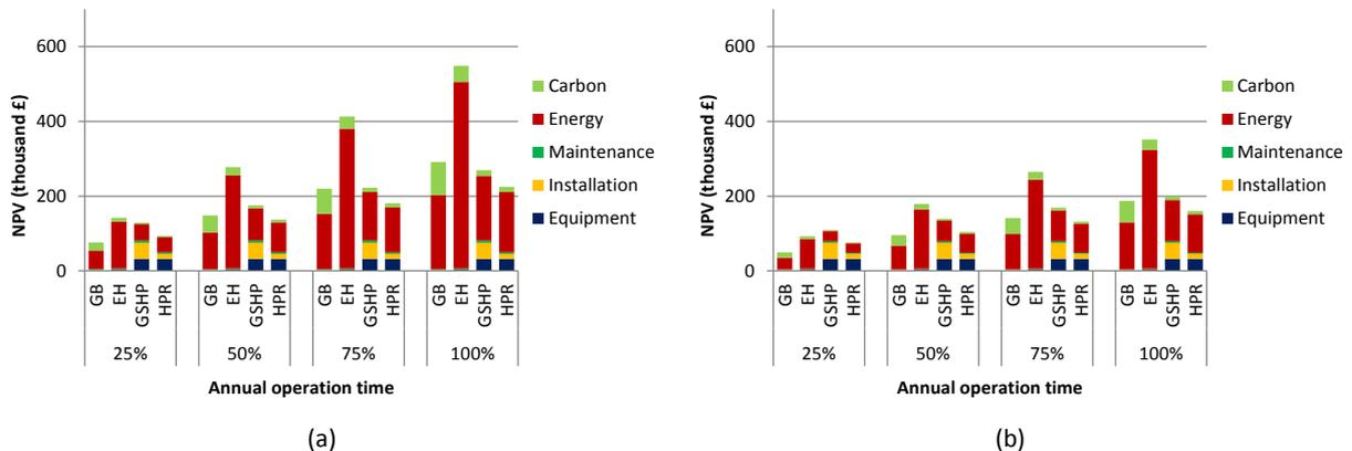
**Figure 40: NPV of different cost components for alternative heating system designs, for discount rates of (a) 3% and (b) 9% (GB = Gas Boiler, EH = Electric Heater, GSHP = Ground Source Heat Pump, HPR = Heat Pump with Recovery)**
