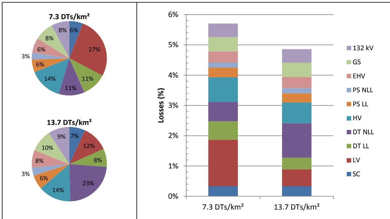
Figure 29: Impact of distribution transformers density on losses in a semi-urban type network
