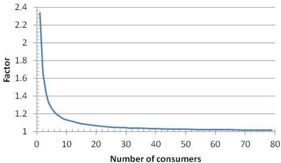
Figure 9: Modelled loss factor for diversified load profiles
