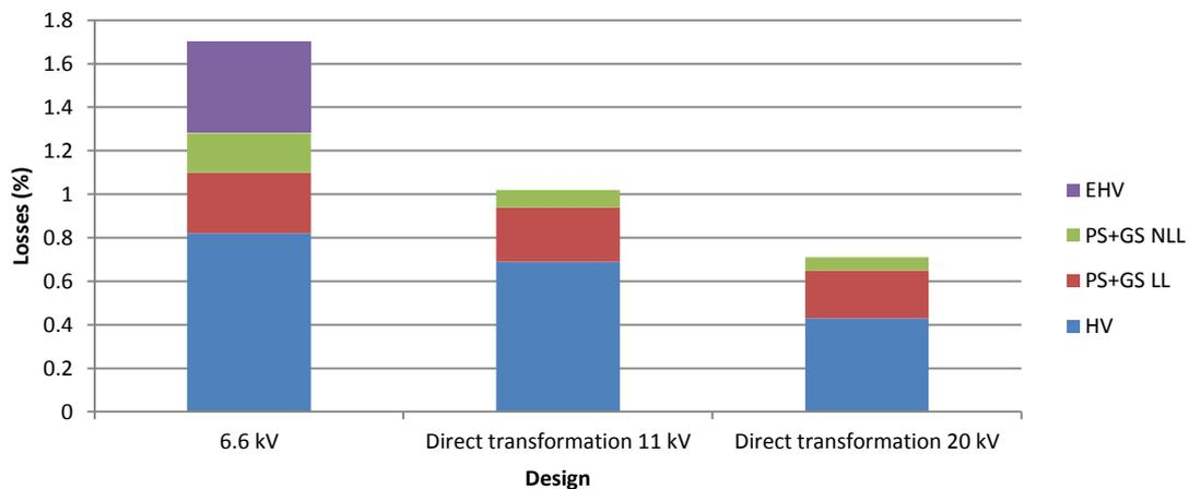
**Figure 32: Losses in distribution systems with various voltage levels; HV – high voltage, PS – primary substation, GS – grid substation, LL – load losses, NLL – no-load losses, EHV – extra high voltage (33 kV)**
