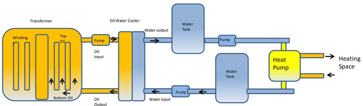
**Figure 37: Concept of heat recovery from distribution power transformers**
