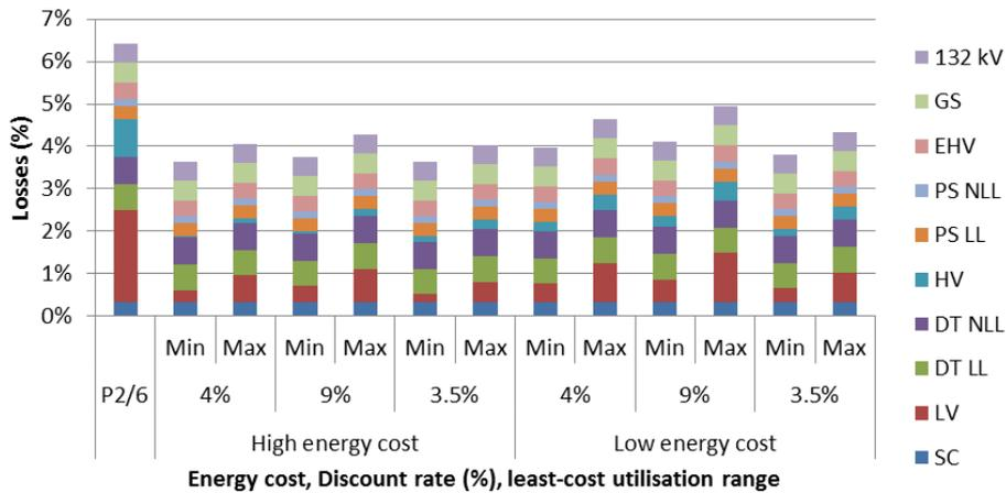
Figure 22: Least cost network design for semi-urban networks
