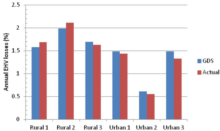
Figure 1: Comparison of actual and estimated losses for GSP models
