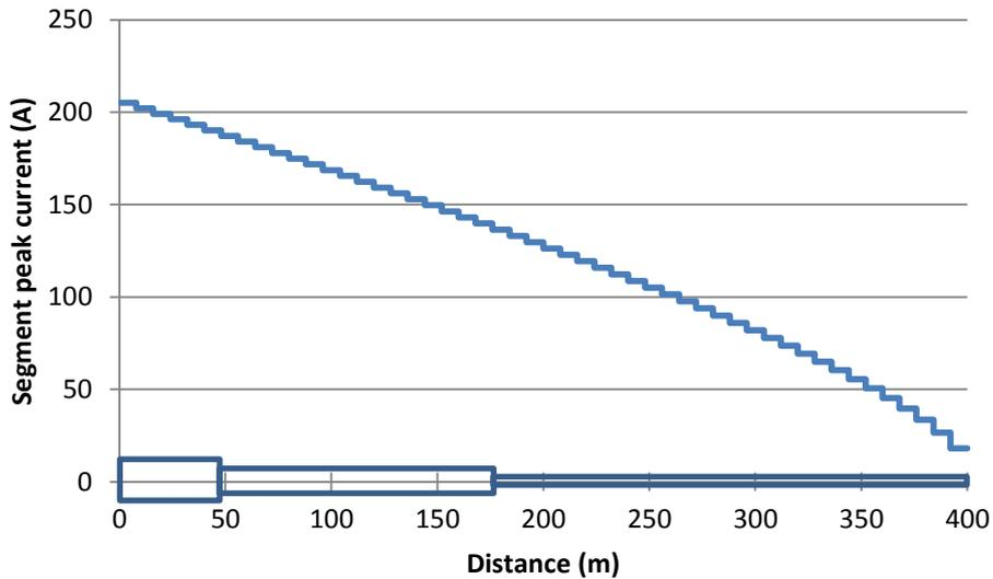
**Figure 36: Distribution of peak currents (not necessarily occurring at the same time) along a feeder of 400 m which supplies 50 customers uniformly distributed along the feeder**
